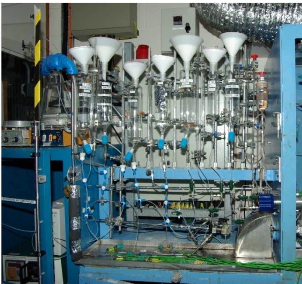
Figure 3-3. Feed vessels for the IP1 rig. The peroxide and water feed vessels are the four towards the left, the quench feed vessel is central, the catalyst and water feed vessels are towards the right and the pX feed vessel is the small one at the right with a red top. Most of the feed vessels also have a parallel burette for feed rate measurement. The funnels and filter papers used to filter feed material are clearly visible. These were left in place during running to protect against the ingress of contamination while allowing material to be pumped without forming a vacuum in the vessel. Blue isolation valves are visible below the peroxide vessels and a network of plastic feed piping with white and blue fittings below these. The isolation valves below the catalyst, quench and pX vessels are metal and have green handles. There is a metallic drip tray below these on the top of the pump cabinet. The feed vessels are in a low-pressure area and are not enclosed. The edge of the (blue coloured) reactor cabinet is visible on the right. The large blue handle protruding through the wall of this cabinet is the control dial for a Pressure Tech back-pressure regulator. The metallic (quarter segment) segment of the drip tray below this handle covers the pipes that house the feed pipes from the pump cabinet (below) to the reactor cabinet. The cabinet to the left houses the degasser unit and a heater control box (which are visible) and additional HPLC pumps which are lower and out of shot. The hot plates on top of this cabinet and conical flask are components of a hot feed system which was intermittently used when feeding catalyst containing lower solubility components. Lagging and trace heating can be seen on sections of the feed lines from this system e.g. the top section wrapped in blue tape and lower sections wrapped in grey foam secured with silver coloured tape. The sections in between have hot water circulation over the feed pipes. The green cabling at the bottom are for thermocouples. Two electrical panels and the trunking of the cabinet extract can be seen at the top left and top right respectively.
