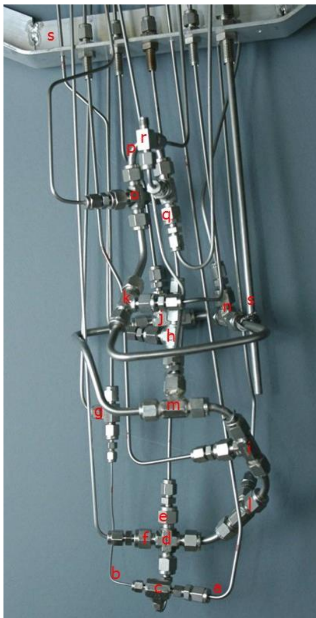
Figure 7-3. Kinetics rig (K5) reactor (Ref. 3 in Figure 7-7) with modified mixer design and 4 oxygen stages. Catalyst solution and pX were fed in (a) \frac{1}{8} " and (b) \frac{1}{16} " tubing respectively to a \frac{1}{16} " Swagelok tee-piece mixer (c). The mixture flowed upwards into a buoyancy mixer (d) constructed from a \frac{1}{4} " cross piece and containing a downwards oxygen/water feed through an \frac{1}{8} " tubing dip-pipe (e) and with a thermocouple inserted through an \frac{1}{8} " line (f). There were thermocouple points on the pX feed line (g) and air/O 2 line (h). There were three additional oxygen/water \frac{1}{4} " tee-piece (i),(j),(k) mixing points in the reactor, fed by \frac{1}{8} " tubing. The first of these (i) had a thermocouple both immediately up (l) and down (m) stream of the mixing point. The other two had thermocouples downstream of the mixing point (n), (o). The reactor flow then passed through a high point (p) and flowed downwards where an up-flow quench (q) was added from an \frac{1}{8} " line. There was a final thermocouple (r) on the line downstream of the quench mixing point. The reactor was attached to supports (s).
