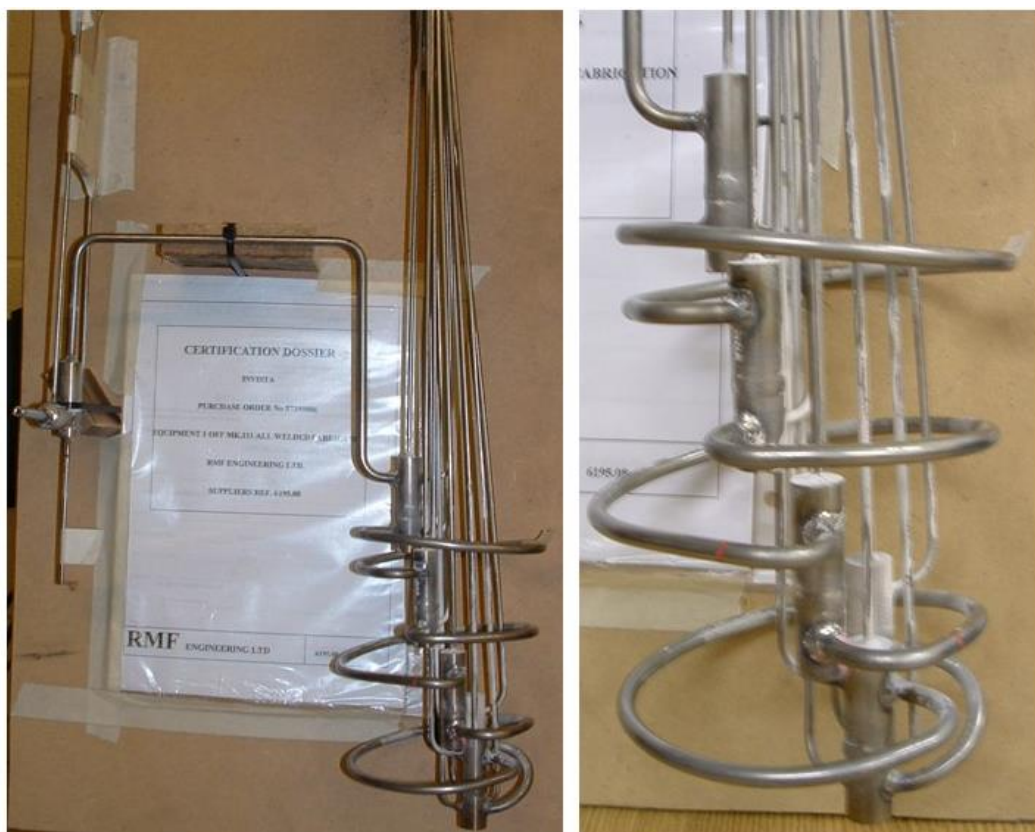
Figure 7-8. The final K5 reactor (Ref. 7 in Figure 7-7), with 4 buoyancy mixers, the first to mix p X, catalyst solution and SCW/O 2 and the other three for further SCW/O 2 staged addition.
