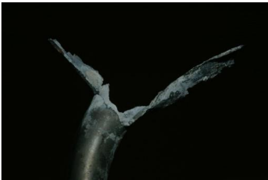
Figure 2-4. A ¼" O.D. pipe after rupture by a pX detonation with O 2 under NCWO conditions. The shredded ribbon structure is typical of a pipe rupture by a detonation event. Note the manganese oxide fouling evident on the interior surface of the pipe which is typical in N/SCWO using manganese based catalysts.
