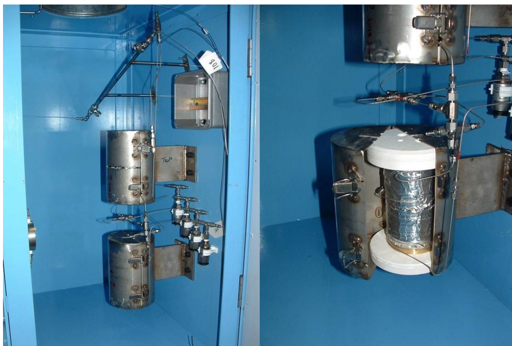
Figure 3-5. IP1 rig reactor cabinet. This photograph was taken when the reactor assembly was under construction; this enables more detail to be seen, as the final assembly was lagged and consequently detail was much less visible. The lower reactor chamber contained the pre-heater; the photograph to the right shows this with the housing open. The assembly comprised a brass block (the brass is just visible above the lower ceramic insulation disc) around which \frac{1}{16} " (and later \frac{1}{8} ") tubing was wrapped and was covered in metallic foil. The whole assembly was covered with lagging and a stainless-steel housing. The reactor was constructed in a similar fashion with \frac{1}{8} " tubing and was located above the pre-heater. There were four pressure transducers to the right of the pre-heater, one on each of the feed lines from the pumps. The mixing cross assembly was just above the pre-heater. In this (early) deployment, the SCW/O 2 feed entered from below and the p X and catalyst entered from the side. There was a thermocouple assembly on the outlet (top of cross). The quench point and cooler assembly can be seen above the reactor. The extraction port is visible in the roof of the cabinet and a vent line can be seen discharging to this on the top left. The back-pressure regulator is just visible on the left.
