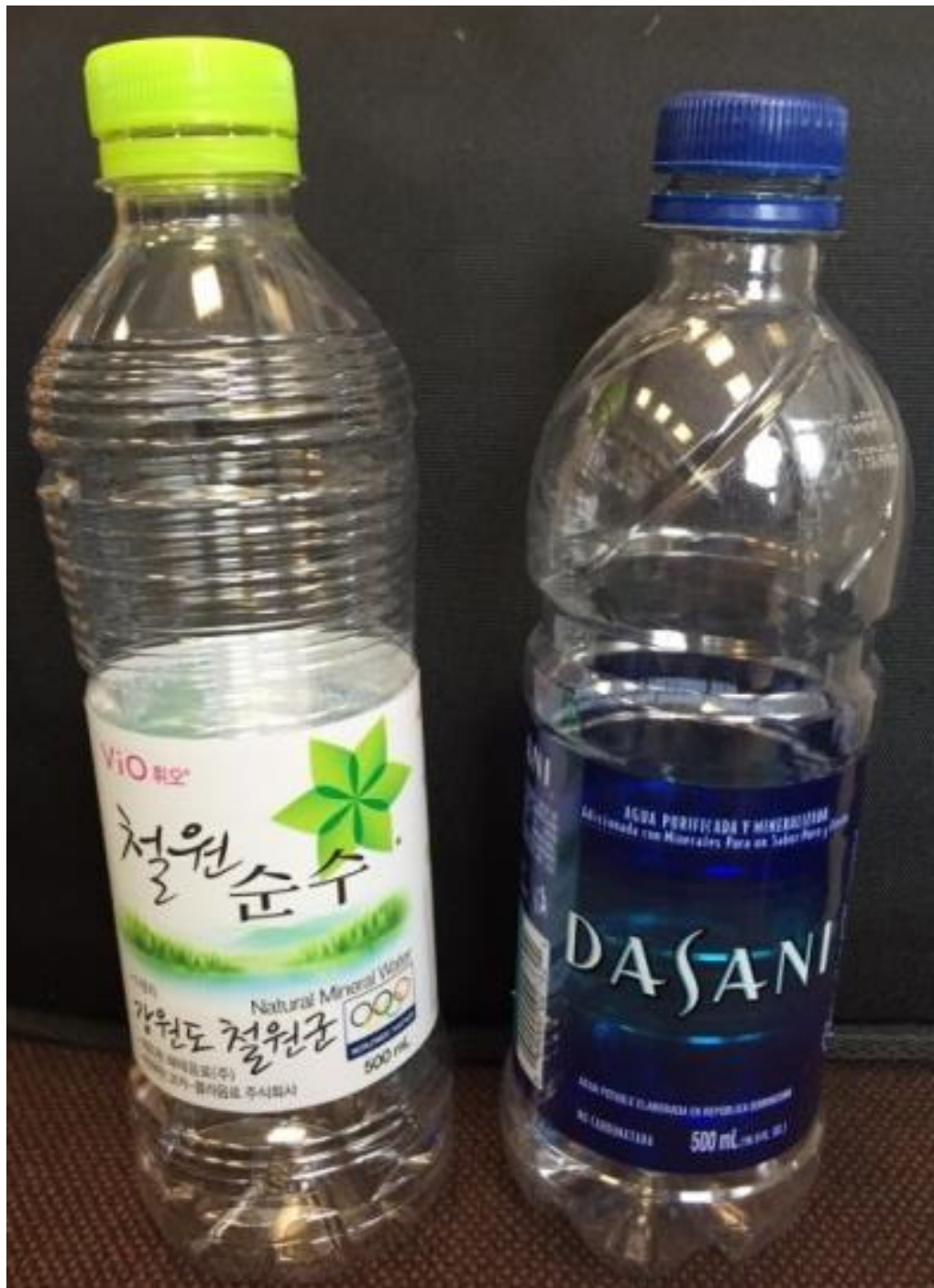
Figure 1-12. A 100 % bio-derived (left) and a fossil derived (right) PET water bottle. There is no loss of bottle quality or functionality in switching from fossil to bio-based feedstocks. The bottles were photographed by the author at the UoN.
