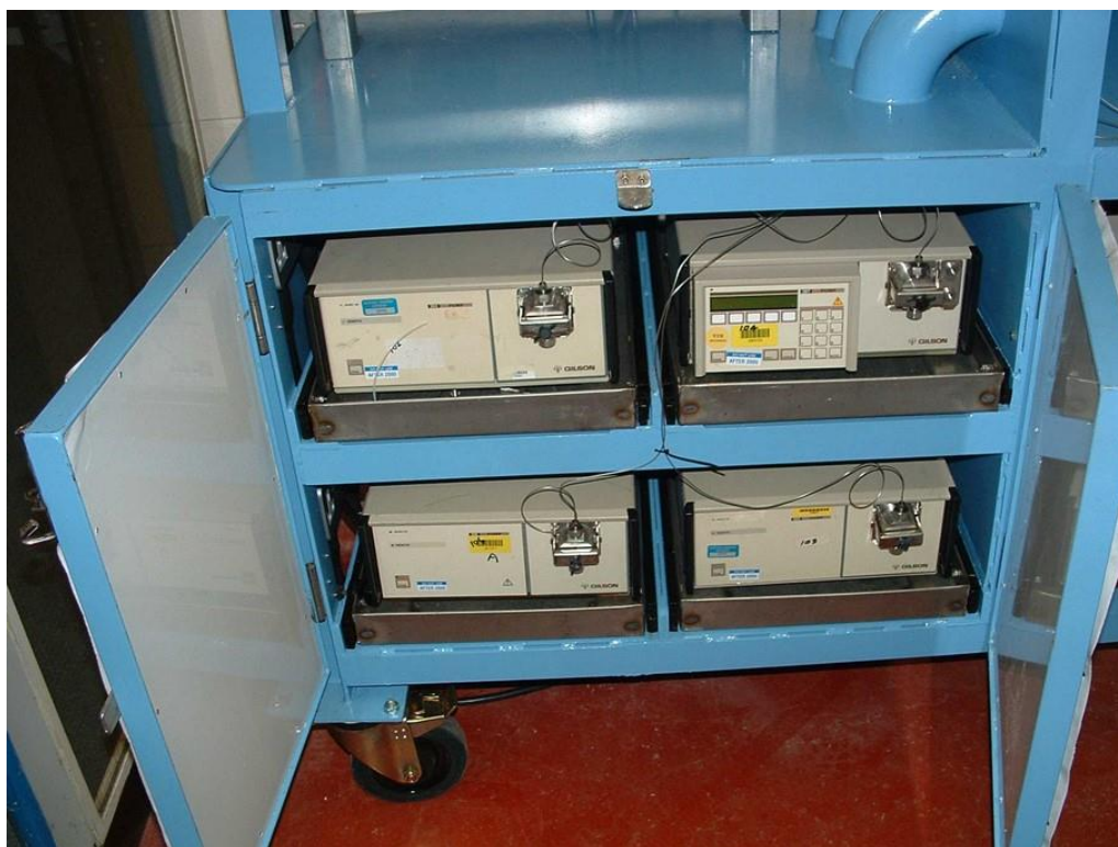
Figure 3-4. Feed pump cabinet on the IP1 rig containing the original four Gilson HPLC pumps. Additional pumps were added later in a second cabinet. Each pump has a stainless-steel drip tray bund. The discharge lines from the pumps pass to the reactor cabinet through the curved blue pipes that are visible top right.
