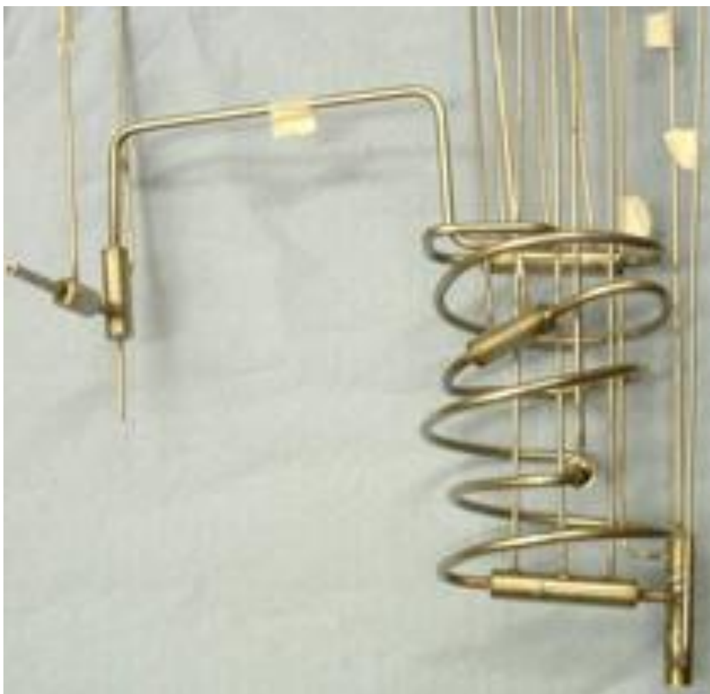
Figure 7-6. The welded reactor (Ref. 6 in Figure 7-7) on the K5 rig. The detail of components can be seen in Figures 7-5. The initial buoyancy mixer is bottom right and has a vertical orientation. Feeds and thermocouples to this mixer enter through the vertical \frac{1}{8} " tubing. The exit from this mixer is to the left through \frac{1}{4} " tubing and immediately enters a tee-piece mixer with a close to horizontal but rising orientation with a O_2/SCW feed and 2 thermocouples entering through vertical \frac{1}{8} " tubing. This is the start of the reaction section. The reactor continues in an upwards spiral of \frac{1}{4} " tubing with 3 further O_2/SCW tee-pieces, feed and thermocouples points and is arranged in this spiral fashion so that it will fit into a sand bath. After the final injection point, the tubing rises vertically to exit the sand bath and then passes through a lute with a high point, designed to prevent back flow of quench into the reactor. It then passes to a quench addition point (seen to the left), that has a vertical orientation, where the caustic quench stream enters through \frac{1}{8} " tubing from below. The exit from the quench mixer is horizontal and passes to a final thermocouple point. Note that all the joints in this assembly that are within the sand bath are welded and all Swaged joint points to this assembly fall outside of the bath.
