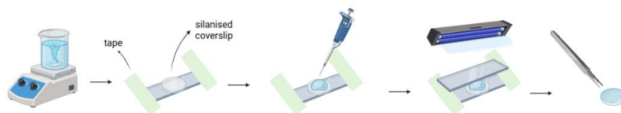
Figure 4.3.13 Schematic representation of the optimised “sandwich” method for producing ALMA hydrogel films with controlled thickness on silanised coverslips.
