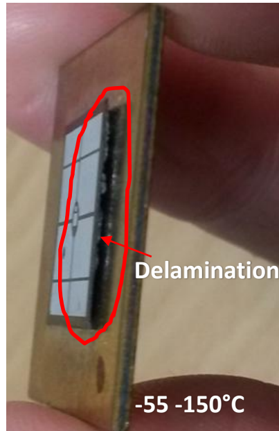
Figure 5- 27: Images of real \text{Sn}_{96.5}\text{Ag}_{3.5} solder joint after thermal cycling for 3000 cycles from -55\text{ }^{\circ}\text{C} to 150\text{ }^{\circ}\text{C}
