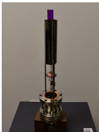
Figure 3.2.3: Photograph of Knudsen cell and crucible that fills with source organic material.
