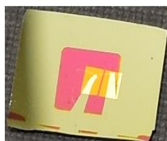
Figure 3.2.8: Photograph of organic field effect transistor of \text{C}_{60} thin film on Si/SiO 2 substrate
