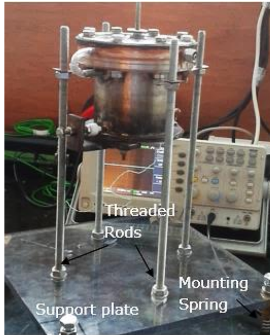
Figure 6.24: Engine support frame
