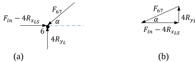
Figure D.8 (a) Free-body diagram of flexure hinge 6, (b) force polygon.
