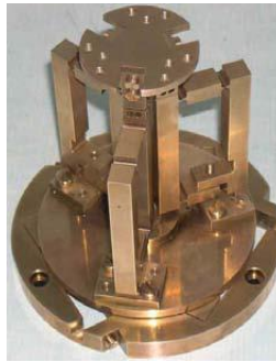
Figure 2.5 Prototype of a 6-DOF micro-stage [4].
