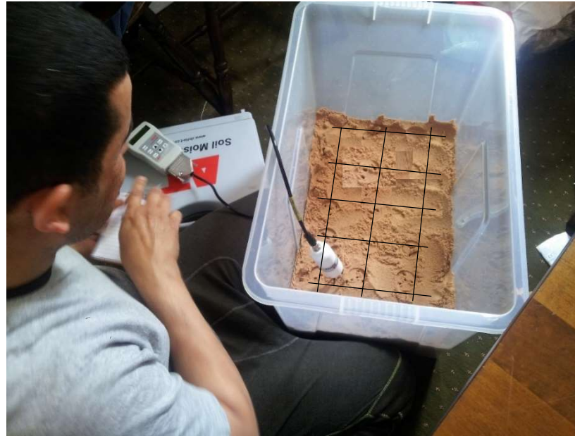
Figure 7.31: Measuring the moisture content of the sand sample over a virtual grid of 3x5, using ML3 ThetaProbe kit.
