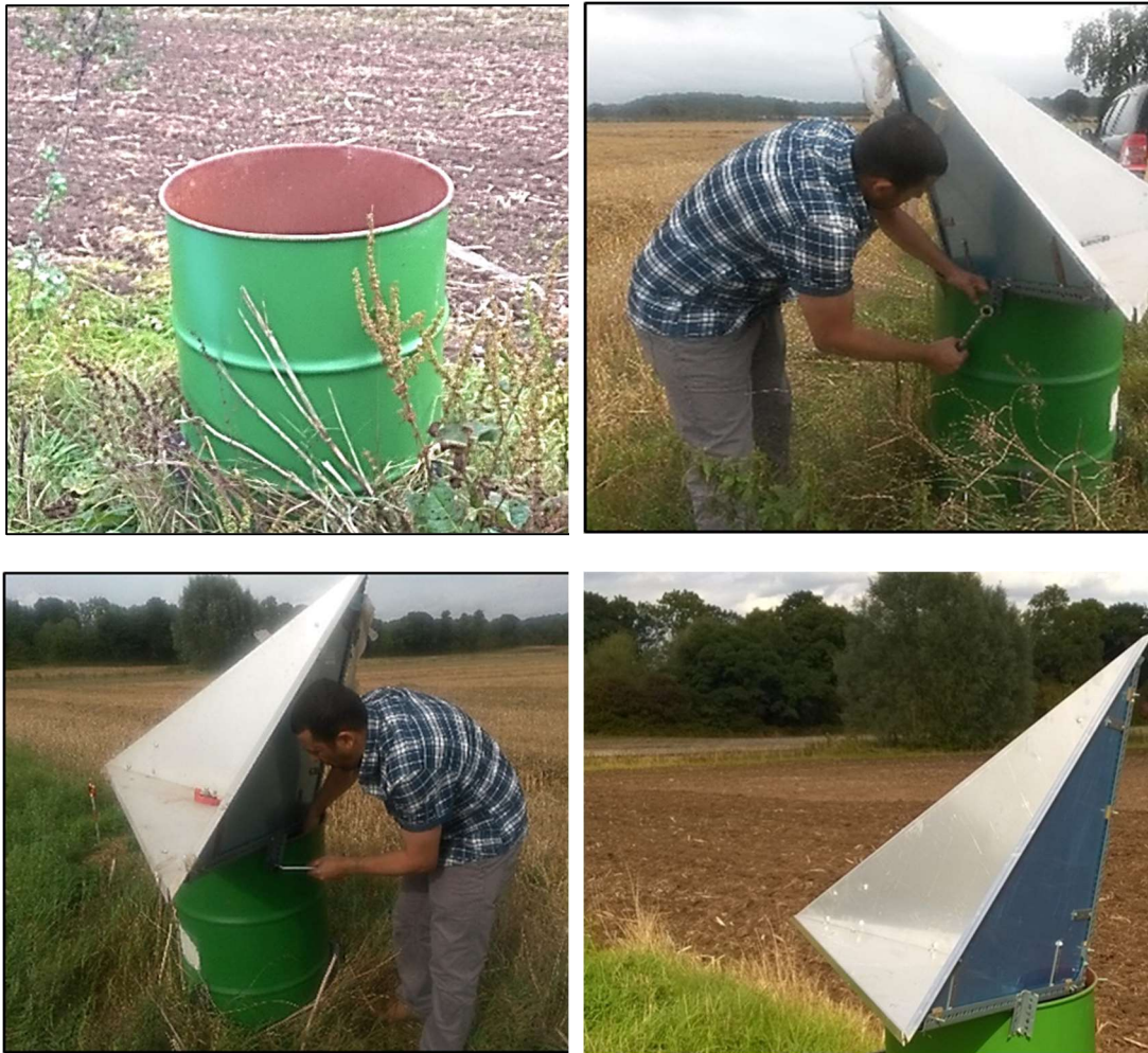
Figure 4.14: The CR is securely fixed on the barrel using screws. The location and orientation of the CR is fixed and cannot be re-oriented.
