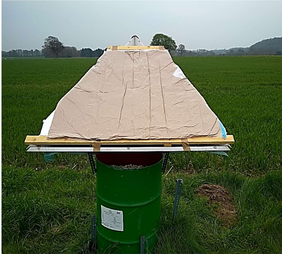
Figure 4.61: The complete layout of the CR with sand cover.
