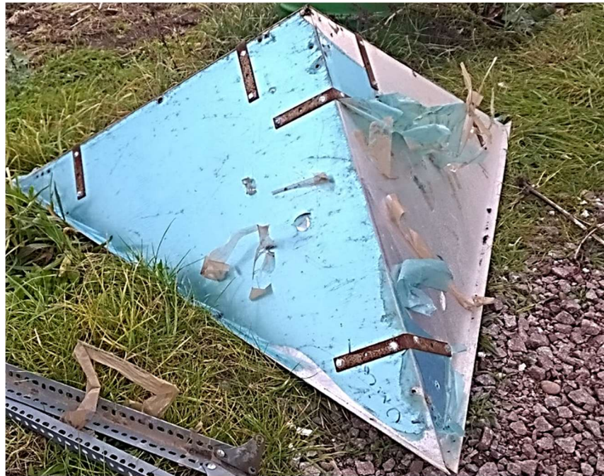
Figure 4.12: Assembled CR. The angle brackets are used to support the faces and maintain the inter-plate orthogonality.
