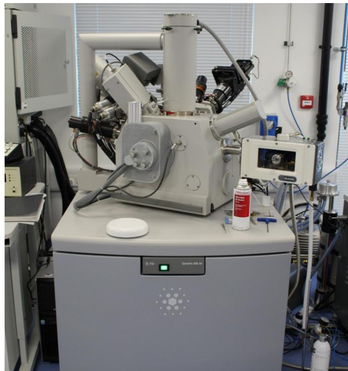
Figure 36: EI Quanta 200 3D Dual Beam FIB-SEM from the nmRC.
