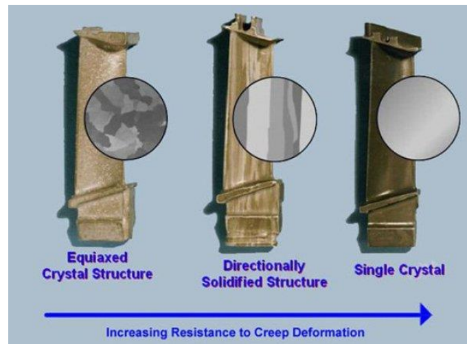
Figure 5: Evolution of the engine blade over the years, highlighting the importance of its crystal structure for improving the performance [17].
