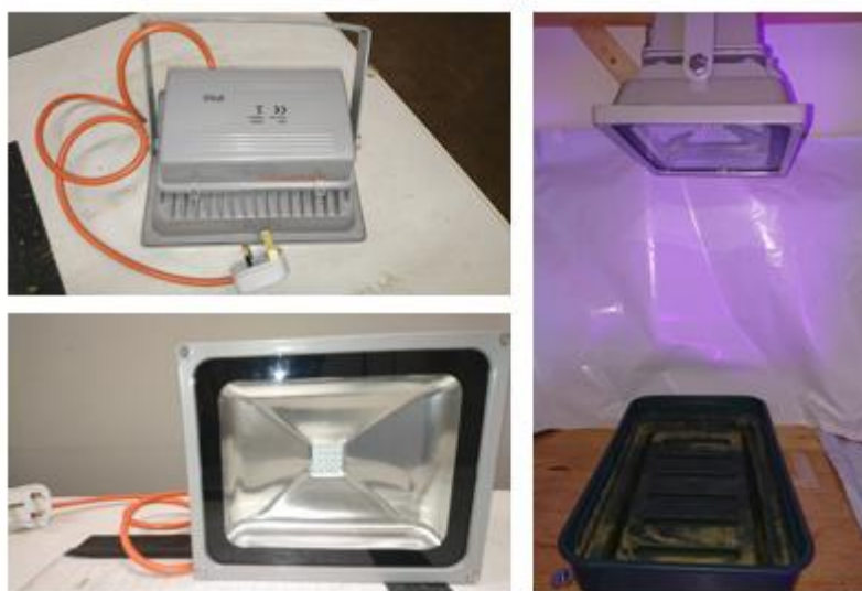
Figure 2.4: The 30 watt LED floodlamps from above, below and in the growth area.
