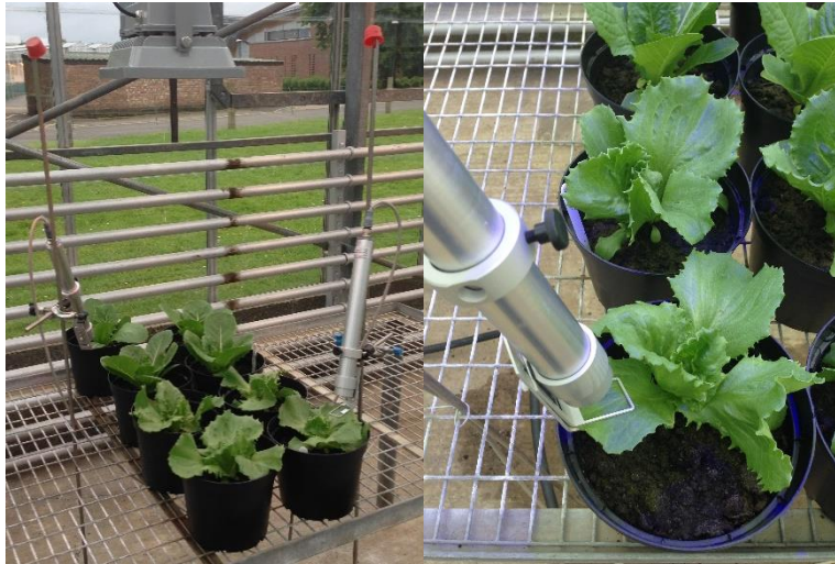
Figure 2.12: Walz MONITORING-PAM Chlorophyll fluorometers for the continuous measurement of \phi\text{PSII} , ETR and NPQ of lettuce leaves.
