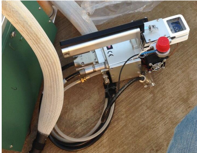
Figure 2.1: The LI-6400XT portable photosynthesis machine measuring head with sun and sky attachment.
