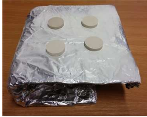
Figure 3.7: Pellets on a tray covered with a boron nitride- coated aluminium foil.
