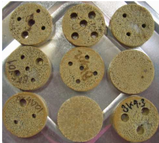
Figure 6.2: 22mm diameter PEEK/NaCl composite samples with assorted drilled holes
