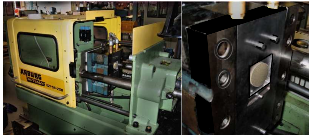
(a) (b) Figure 6.6: (a) Moulding machine used to integrate the porous and solid part and (b) the mould cavity with PEEK/NaCl “composite” insert
