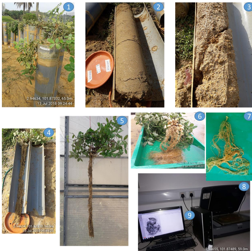
Figure 3.7.4: Extraction of roots from the PVC columns; 1-plants in PVC columns, 2- opening the column, 3-soil removal by water, 4-debris and soil removal, 5-appreciating the rooting depth, 6- more cleaning and debris removal, 7-suspending the roots in the Plexiglas trays ready for scanning, 8- scanner machine and 9- computer with WinRhizo Pro software.
