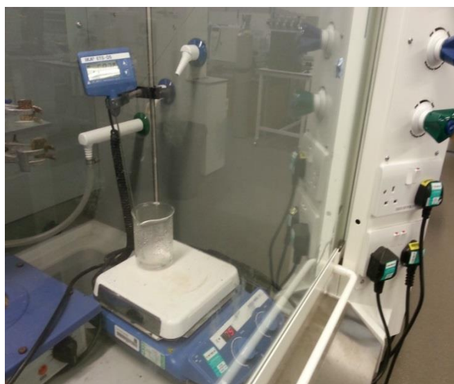
Figure 3.1. Sorbents preparation by co-precipitation method using a hot plate magnetic stirrer inside a fume cupboard.
