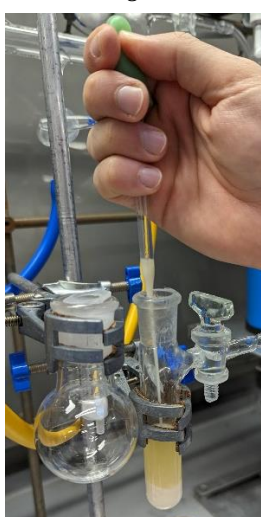
H: filtering of alumina
