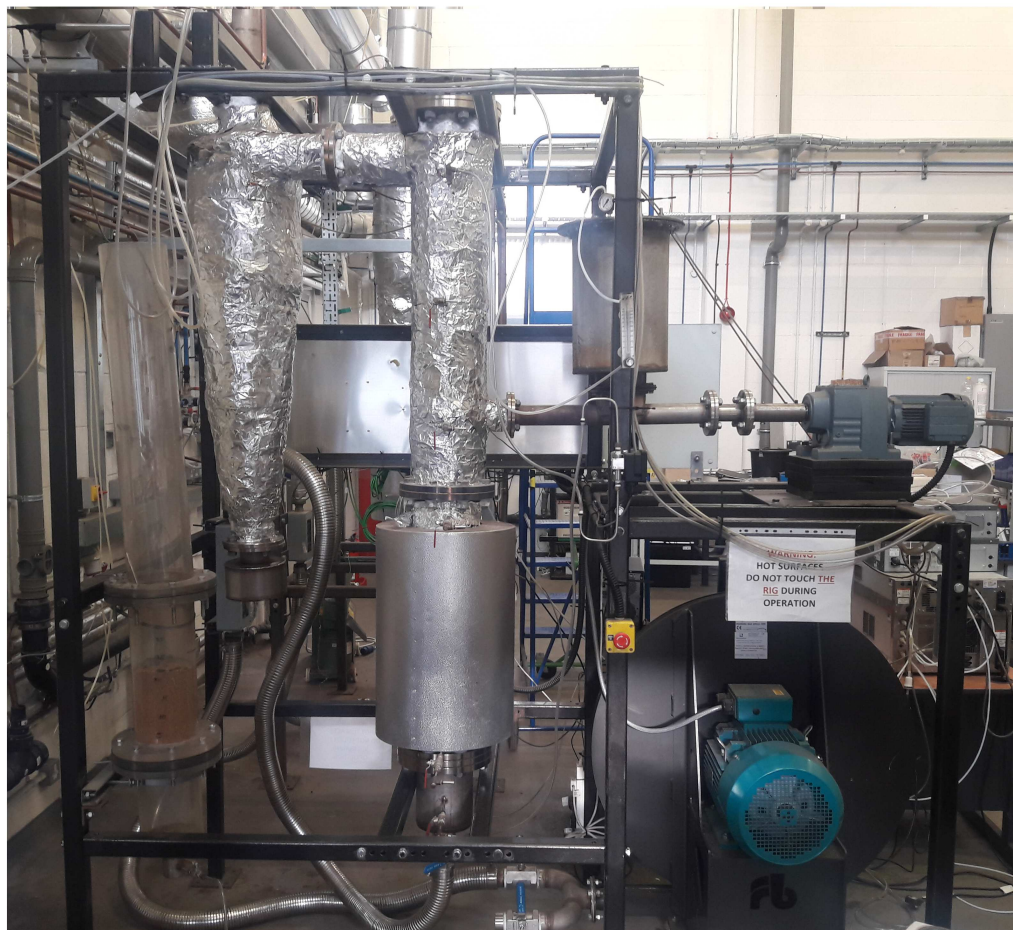
Figure 3-14: Schematic diagram (top) and photo of pilot-scale (bottom) BFB combustor.
