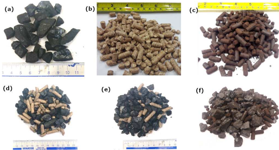
Figure 3-18: Selected samples of pure fuels and blends used in the BFB combustion experiments, (a) bituminous coal (BC), (b) commercial wheat straw pellets (STW), (c) in-house manufactured spent coffee ground pellets (SCG), (d) BC blended with STW at 40 wt%, (e) BC blended with STW at 15 wt%, and (f) BC blended with SCG at 40 wt%.
