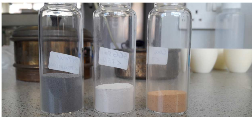
Figure 3-3: Sieved ash samples of wheat straw (left), spent coffee grounds (middle) according to BS/EN/ISO 18122:2015 and bituminous coal (right) according to BS/ISO 1171:2010.
