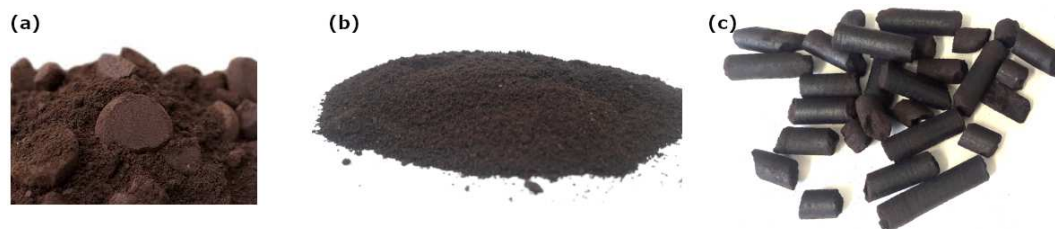
Figure 3-2: SCG pellets manufacturing progression, (a) as received (moisture content > 60 wt%), (b) moisture content \sim 15 wt%, and (c) manufactured SCG pellets.
