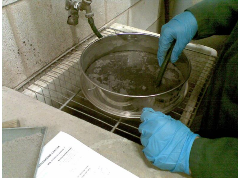
Figure 3.11: Washing of filler on 63 \mu m sieve
