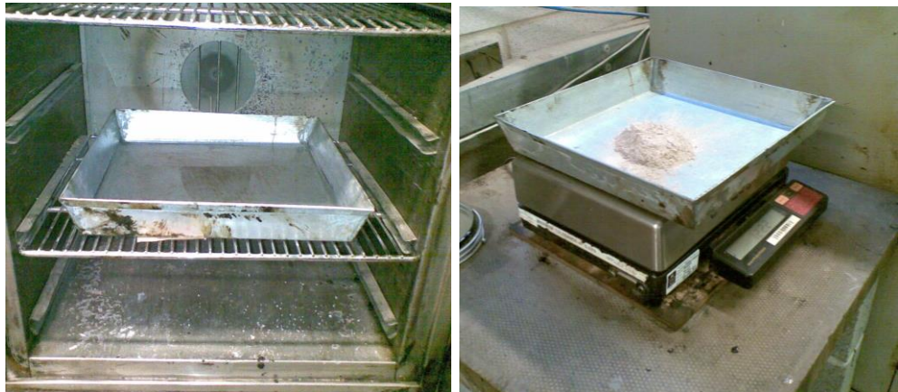
Figure 3.12: Drying and weighing of fillers after washing on 63 \mu m sieve
