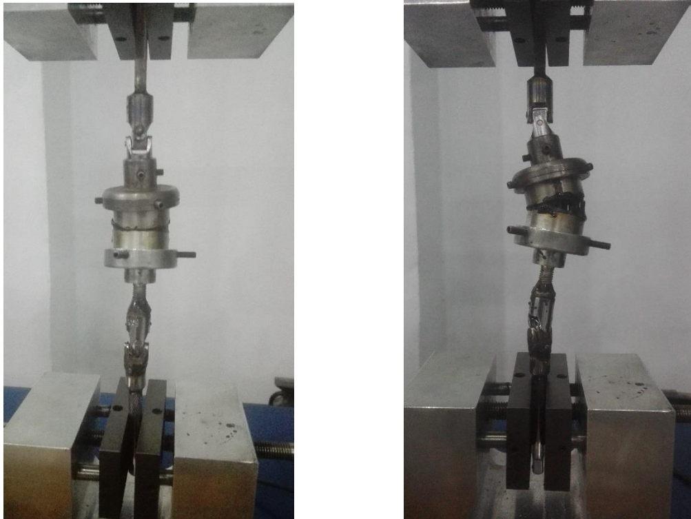
Figure 7.6: Direct pull off testing assembly during and after test
