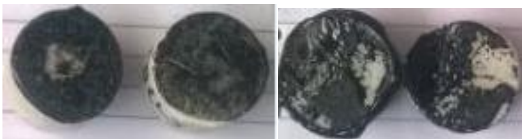
Figure 7.22: Failure at interface of binder and substrate
