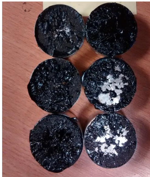
Figure 6.6: Failure surface of Gs mastic after 20 hr ageing
