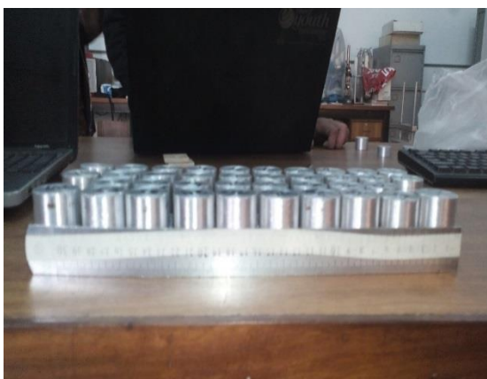
Figure 7.20: Curing of butt-jointed specimens
