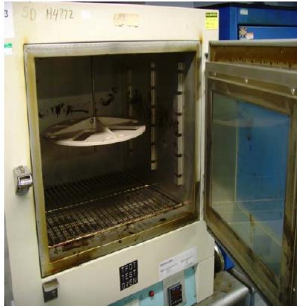
Figure 2.7: Typical TFOT oven (Wu, 2009)
