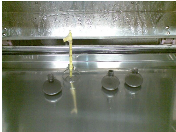
Figure 3.9: Pycnometer left in water bath
