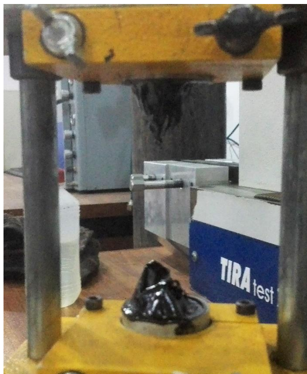
Figure 7.19: Central cavitation for lower aspect ratio
