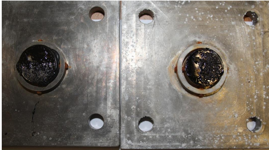
Figure 6.2: Specimen after pull off testing (method 1)
