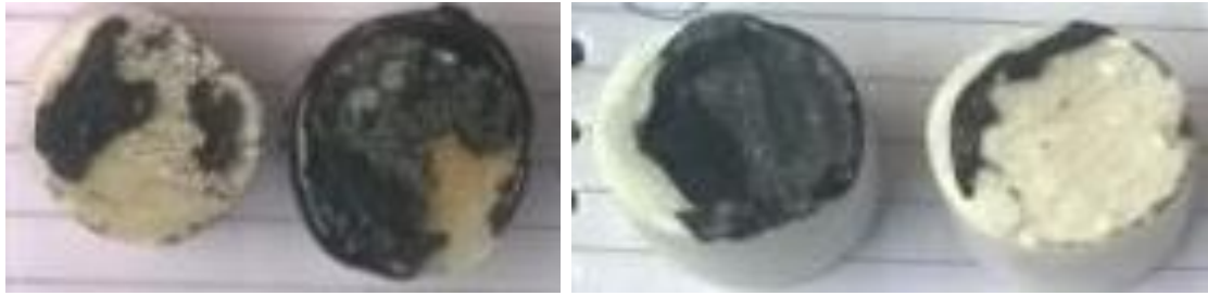
Figure 7.23: Failure due to dust coating
