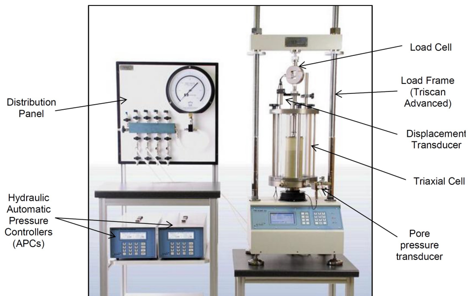
Fig. 4.38 Triaxial setup used for CU test in M_{90-10} mixture, provided by VJTech.
