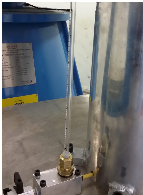
Fig. 6.4 Graduated measuring cylinder (standpipe) for the determination of the water volume extracted from the soil.
