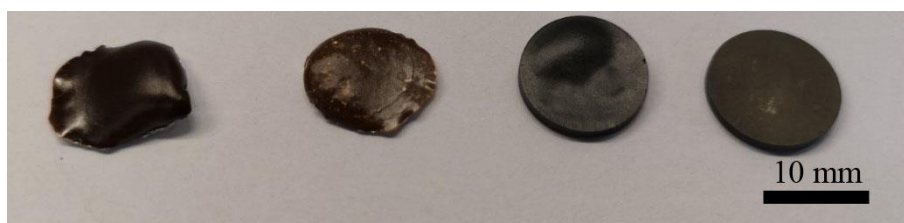
Figure 5-12 Photo of pure PEEK, Ag-PEEK, GNT-PEEK and FGAgT-PEEK composites after 400°C annealing.
