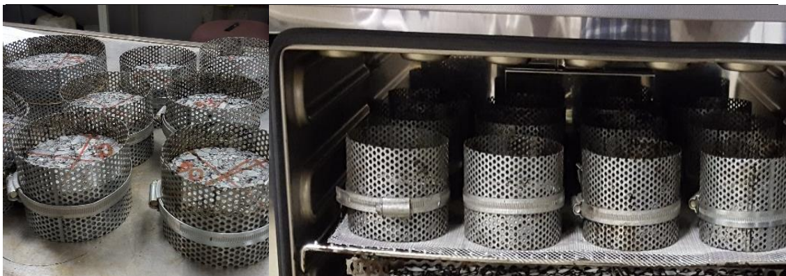
Figure 6-3 Sample ageing procedure involving encapsulating in steel cages.
