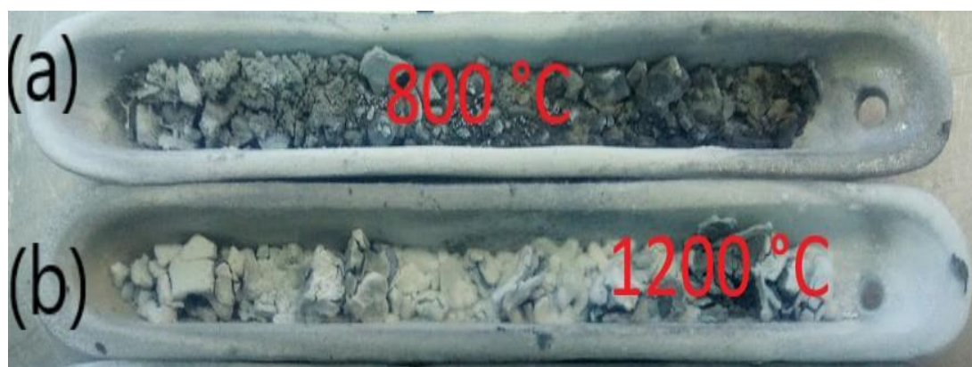
Figure 15 BNNTs produced under ammonia and nitrogen gas atmosphere at temperatures (a) 800 °C and (b) 1200 °C.
