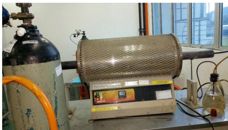
Figure 13 Tubular furnace used for annealing process of BNNTs.
