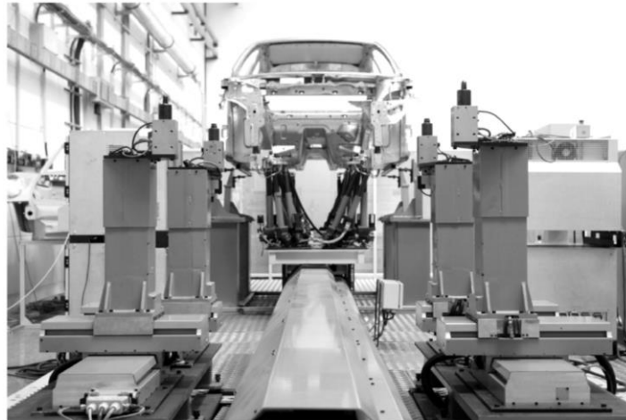
Figure 43. Reconfigurable cell for BiW assembly. Underbody tooling (centre) reconfigures for different models. Bodyside tooling (left and right) reconfigures for different variants to suit each model (Soetebier et al. 2011)
