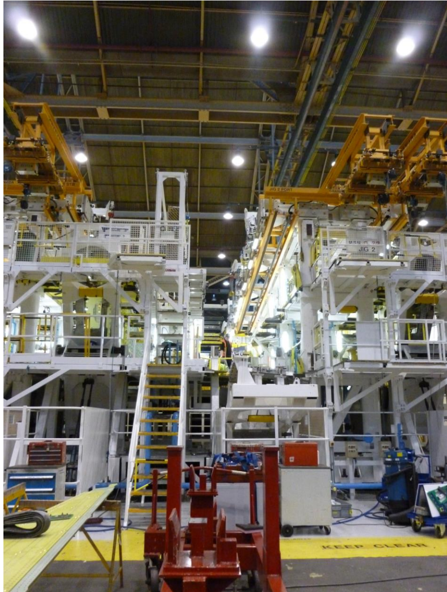
Figure 7. Image of fixture taken from ground floor. Fixture height is approximately 8m. Note overhead cranes used to load wing structure
