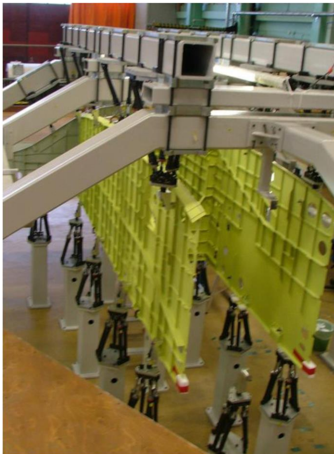
Figure 40. Steward platforms are mounted to a modular structure to provide flexible fixturing for multiple geometries of a UAV. The tooling can be disassembled and reused elsewhere (Kihlman & Engström 2010)
