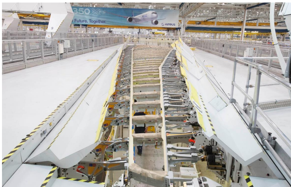
Figure 10. Image of an A350 assembly cell showing ribs assembled to front and rear spars. The ladder structure is lowered onto an AGV and moved to the next cell for cover drilling using a gantry machine (top left) (Airbus S.A.S 2015b)
