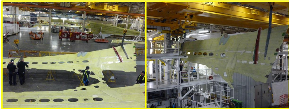
Figure 9. Skins deflect out of tolerance during loading (left) which then have to be manipulated manually into position in the fixture (right)
