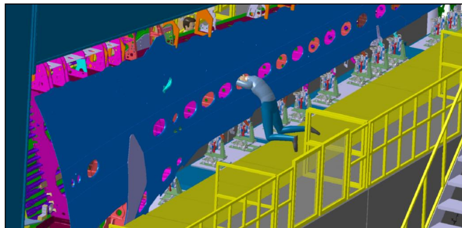
Figure 130. Access for fastening upper cover is through portholes in lower cover
