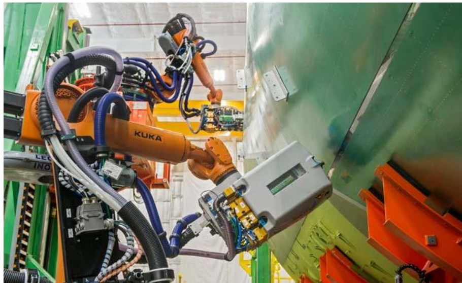
Figure 41. 777 automated fastening system using industrial robots and mobile platforms (Flight Global 2015b)
