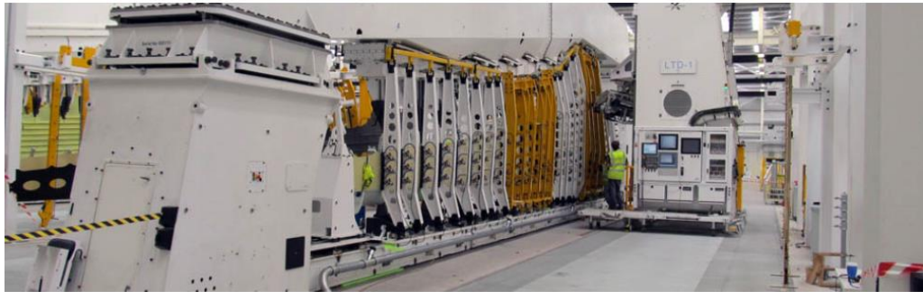
Figure 38. Wing assembly system with mobile automated drilling and bolting system (Electroimpact Inc. 2015; Krejci 2011)
