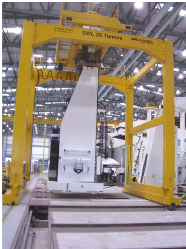
Figure 37. Composite Automated Wing Drilling Equipment (CAWDE). The drilling system is moved between fixtures without reducing accuracy (Hempstead et al. 2006)
