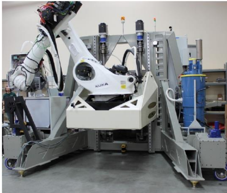
Figure 39. Mobile robot platform for aerospace assembly (Adams 2014)
