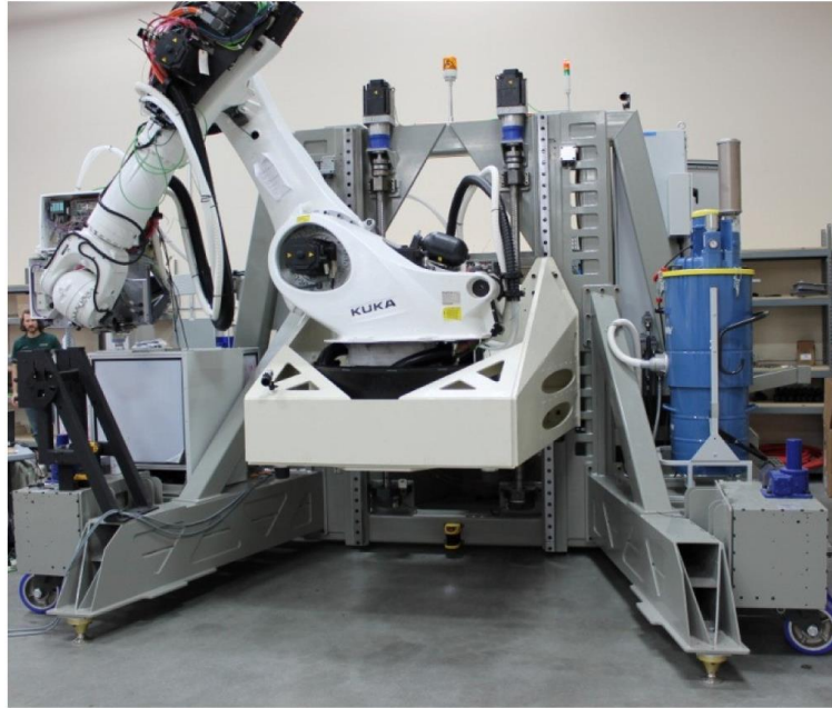
Figure 121. ElectroImpact mobile robot which could be used for reconfigurable assembly (Gray et al. 2013)
