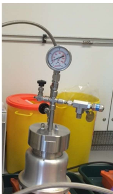
Figure. 17 Setup for the samples enclosed in a CO gas chamber for CYP450 content determination.
