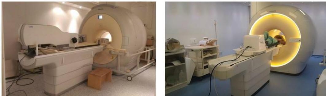
Figure 8-1: A. Exercise set up in the 3T Philips Achieva using the MR compatible supine cycle ergometer (Lode B.V, Netherlands), B. Exercise set-up now available in the 3T Philips Ingenia wide bore scanner using the Ergospect diagnostic pedal system.
