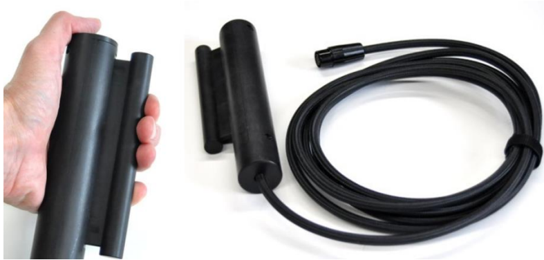
Figure 7-15: The handgrip dynamometer used in this fMRI study. The device is MR compatible and communicates with an interface box via an optical fibre cable. (Images sourced from ' http://www.curdes.com ').
