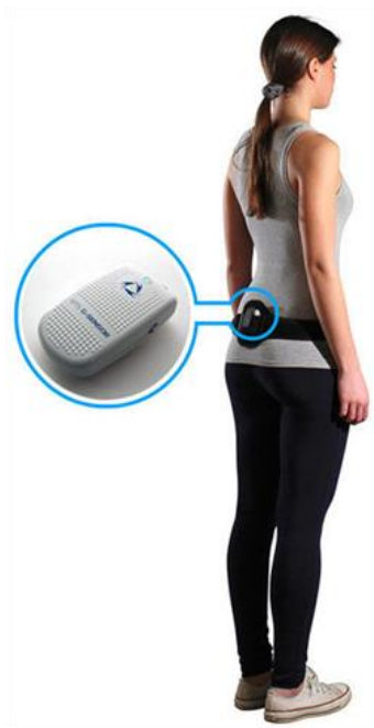
Figure 5.2- An example of the G-Sensor 2 placement. Image taken from Ruben et al 385
