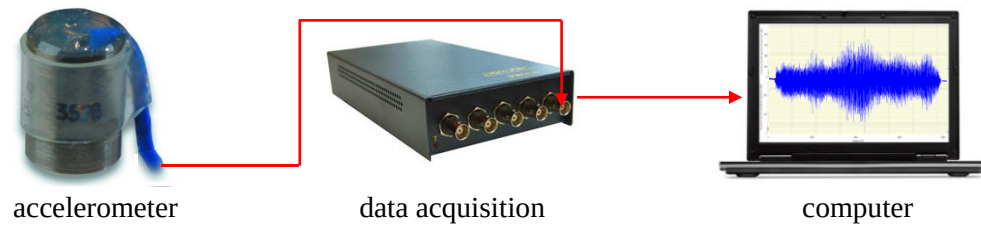
Figure 3-10. Measurement chain schematic for workpiece vibration in machining.
