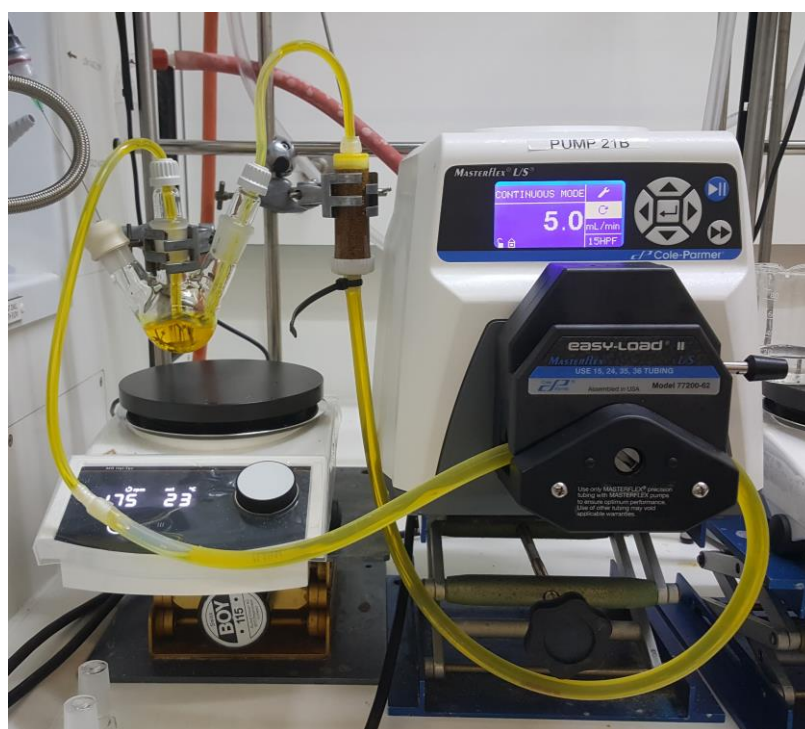
Figure 6: Typical flow reactor setup for synthesis and use of the monolithic dioxypyphosphorane 97 . Three necked round bottomed flask contains reagents in solution. Empty column chromatography column contains monolithic polymer and molecular sieves.
