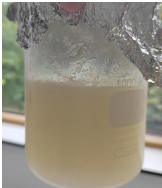
Figure 8. Collagen extraction with dry flocs form of fish swim bladders after 2 days salt precipitation of the collagen.
