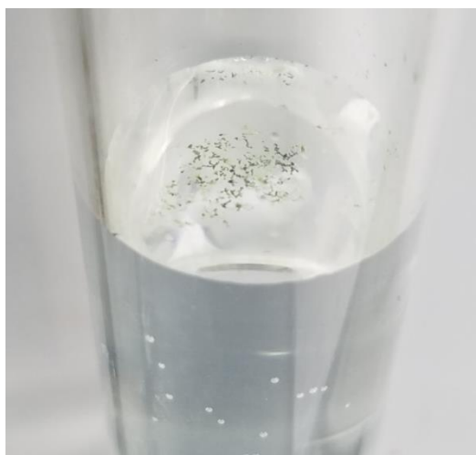
Figure 4.4: Green solids found after the trial of \text{CuCl}_2 extraction by ethyl acetate and Htta. The solids were found floating in on the surface of the solution after two hours of treatment
