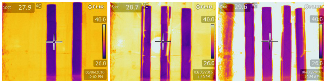
Figure 3.39 Surface temperatures recorded for DBT-WBT of 9,10 and 11°C; and different ceramic arrangements
