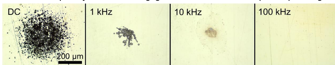
Fig. 4.2. Effect on the workpiece surface at different excitation frequencies for a consistent total of 12 mC anodic charge transfer.
