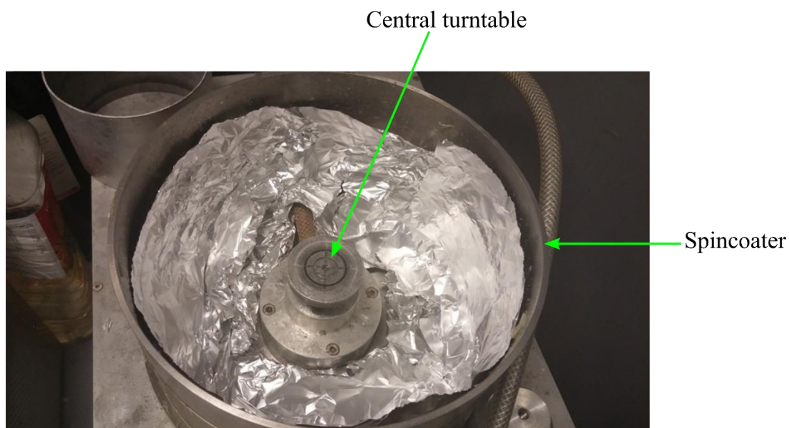
Figure 3. 3: Photo shows the spin coater used in this experiment. The substrate that is to be coated is positioned in the central turntable and it is held on place by suction of vacuum pump.
