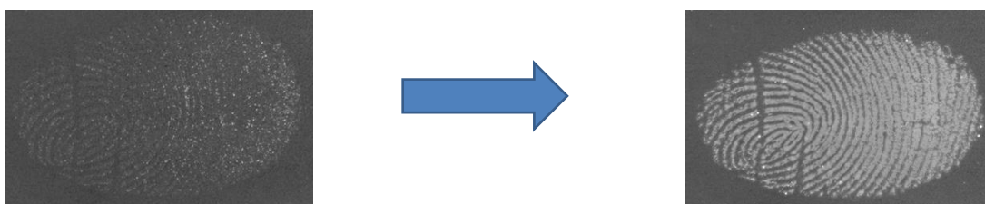
Figure 4. 11: An example of fresh sebaceous fingermark deposited at the time t = 0 minutes and fumed on PtBMA surface after 333 minutes.
