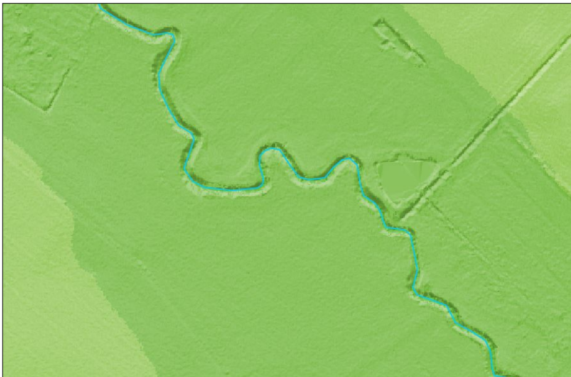
Figure 3.2: Model DTM with hill-shading applied and river centreline drawn
