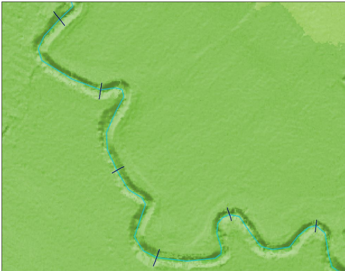
Figure 3.3: GIS polylines representing cross-sections through the river channel
