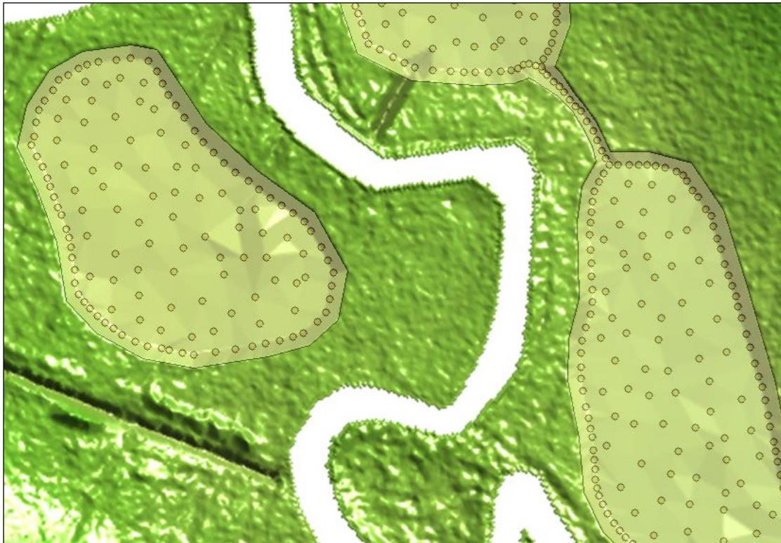
Figure 3.9: Creation of wetland ponds using polygons and points to create a TIN, modifying the DTM (shown)
