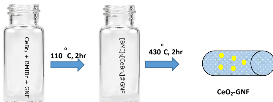
Figure 18 Schematic illustration of ionic liquid mediated preparation of nanocomposite of CeO 2 nanoparticles in GNF (CeO 2 -GNF) from CeBr 3 .xH 2 O precursor.
