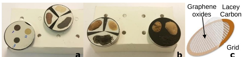
Figure 2-5. Samples for various electron microscopic techniques, (a) SEM samples obtained by casting way, (b) SEM samples prepared by freeze dry and (c) TEM sample grid [194]
