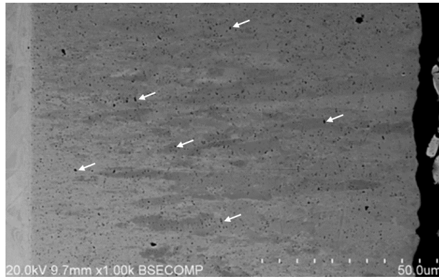
Figure 2.44 BSE image of a typical microstructure of Ni/Al 2 O 3 composite coating. The pointed locations are embedded Al 2 O 3 particles [146].
