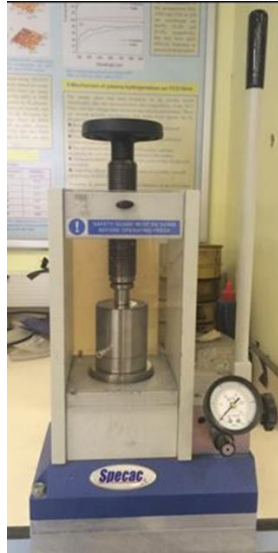
Figure 3.4 Image of the pellet press used to press the powder mixtures of Al and \text{ZrO}_2 into a 20 mm diameter pellet.
