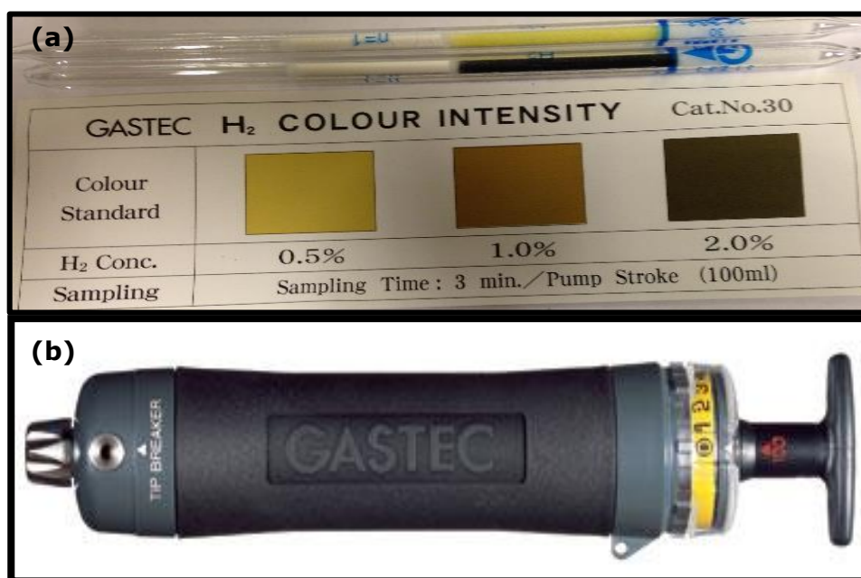
Figure 3.11 – Hydrogen gas detector (a) Hydrogen gas tube detector, (b) GASTEC sampling pump.
