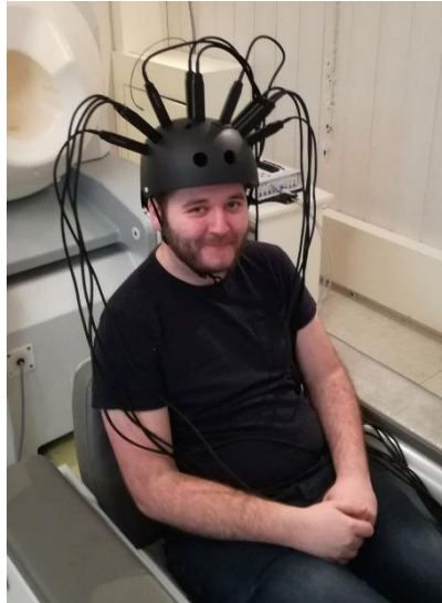
Figure 4.7: Adult bike helmet. The modified adult bike helmet with sensors held in place with slots cut into the helmet. The thickness of the helmet allows the sensors to be held still and at a fixed orientation during scanning.
