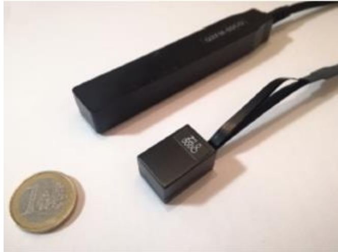
Figure 6.1: Gen-1 vs. Gen-2. Comparison of the two generations of QuSpin OPM sensors with a coin for reference. Adapted from Osborne et al. (Osborne et al., 2018).
