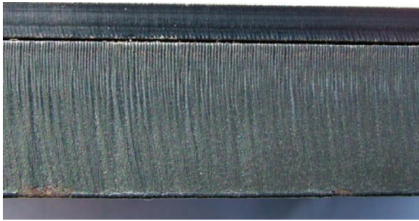
Figure 2.31-Typical of mild steel cut edge produced by CO 2 / oxygen cutting [13].
