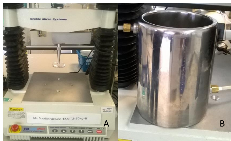
Figure 4: Texture analyser equipment setup used for chocolate meltdown measurement (A) fitted with perspex probe, and stainless steel vessel (B) used for the analysis of meltdown.
