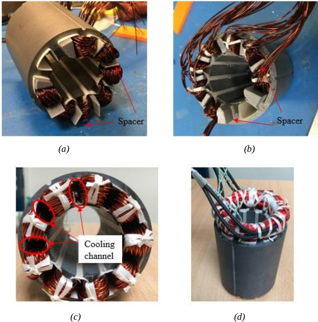
Figure 5-2: Stator core with winding and details of the cooling channel
