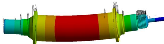
Figure 4-34: The first bending mode of rotor assembly
