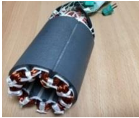
Figure 5-10: Analysed stator / winding assembly
