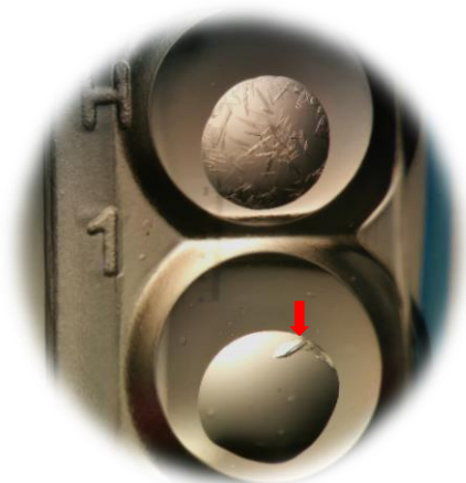
Figure 5.5 Crystals of pyocin S3 DNase-Immunity protein complex formed within 5 mins of setting up crystallographic screens.
