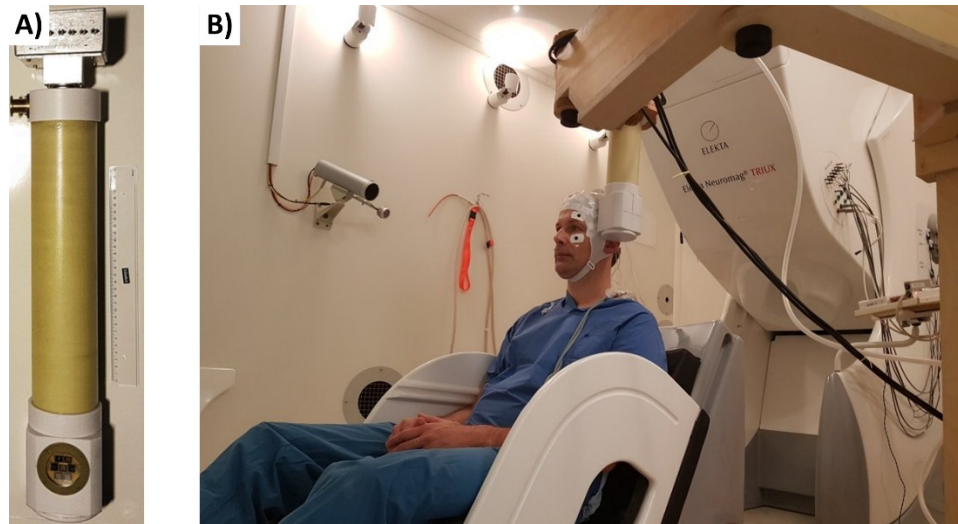
Figure 3.1: A) 7-channel HTS SQUID array in a cryocooler, developed at Chalmers University in Gothenburg. B) On-scalp MEG recording system captured at the Swedish National Facility for Magnetoencephalography (NatMEG). Both adapted from Pfeiffer et al., 2019.
