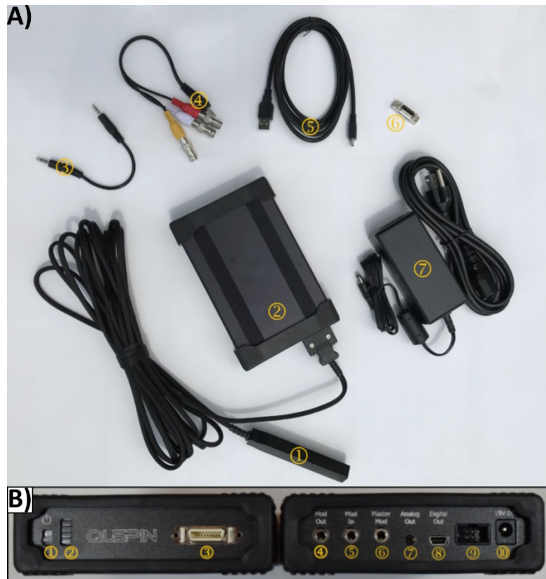
Figure 3.17: QZFM electronics package. Panel A) includes : 1) QZFM sensor head, 2) electronic box, 3) 6.5mm aux cable, 4) 6.5mm BCN splitter cable, 5) micro-USB to USB cable, 6) Shorting cap to protect the sensor head electronics, 7) 19V power supply. Panel B) shows the sensor control electronics box. Includes: 1) Power switch, 2) LED sensor status indicators, 3) sensor head connection port, 4) modulation signal outlet, 5) modulation signal inlet, 6) master modulation outlet, 7) Analog signal outlet, 8) micro-USB port, 9) DUNNO, 10) 19V power adapter inlet.
