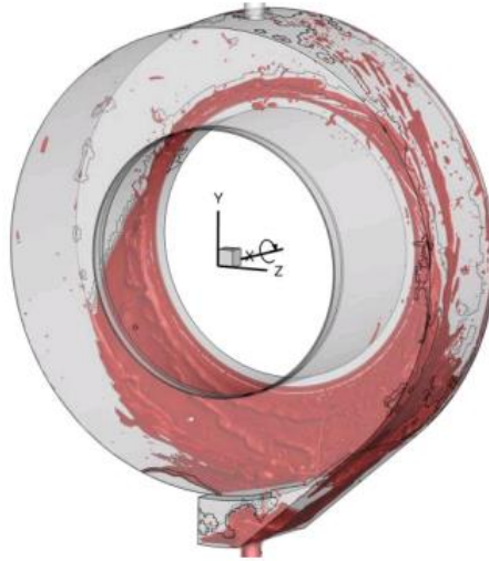
Figure 2.12 – Bearing chamber simulation using adaptive meshing , iso-surface of oil volume fraction \alpha_o = 0.25 [34]
