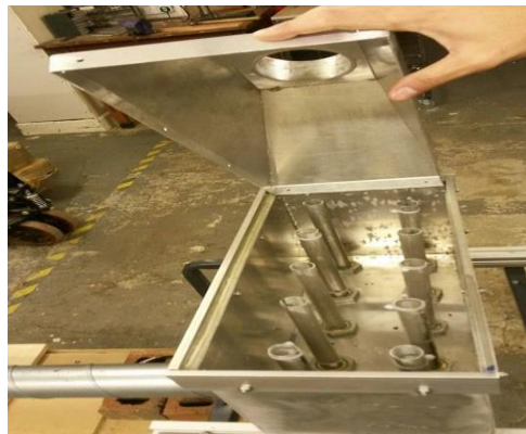
Figure 8.6. Internal view of reactor showing perforated diffuser pipe allocation The tubes are connected to an external manifold (12) to equalise airflow to each tube, with the top end of the tubes sealed in order to achieve the sufficient internal pressure, providing air flow laterally to the absorbent (9). The
