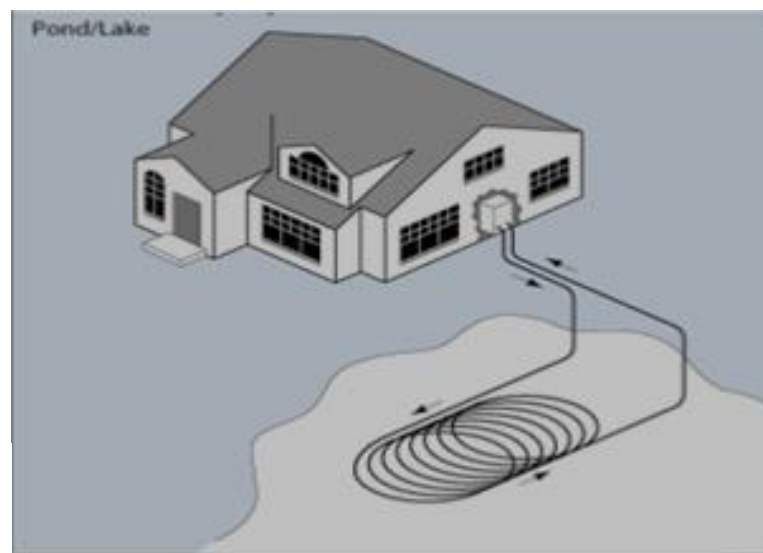
Figure 3.8. The Surface-water heat pump system (WBDG, 2016).
