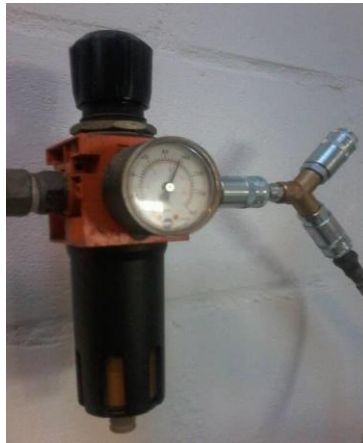
Figure 9.17. In-line pressure gauge to measure the air
