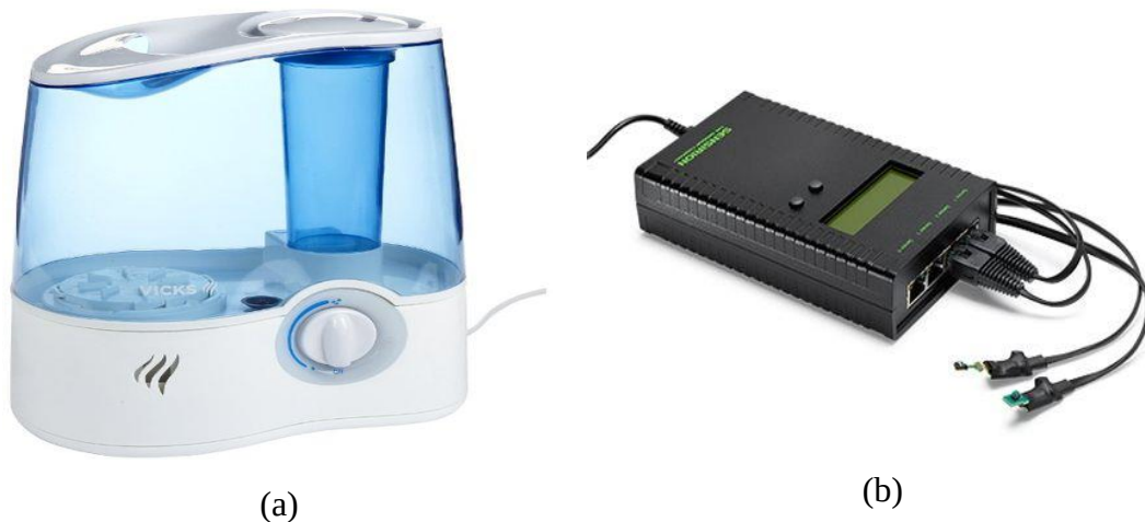
Figure 9.14. The 3.5 ltr humidifier and humidity sensors measurements tool The sensors are positioned at the tip of the probe, which is secured against damage by a membrane filter. The electric power consumed by the air heater and the blower fan (Figure 9.16) was measured using digital power meter
