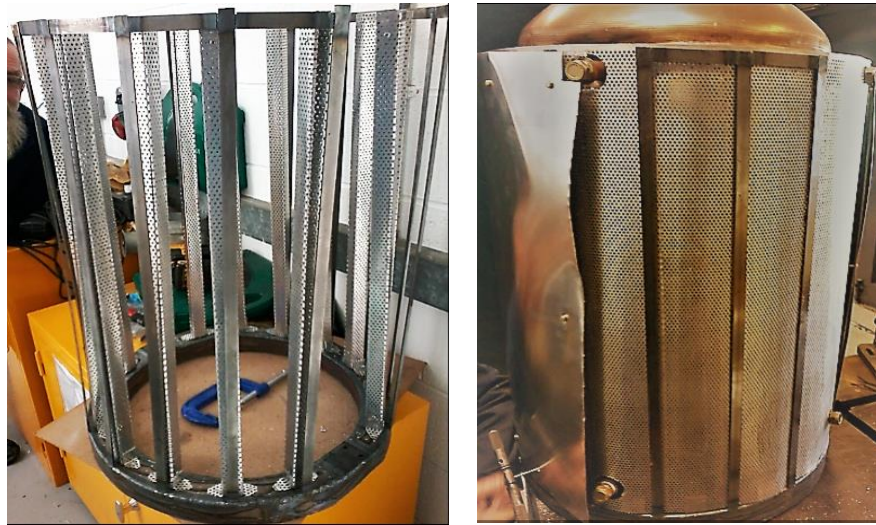
Figure 9.3. The fabrication and rigged of proposed thermochemical jacket A DHWT of 200 litre capacity which is made of Bare copper is used as depicted in Figure 9.2 and Figure 9.3. The outer surface of the bare DHWT and the jacket are twisted by perforated aluminium sheets as shown in Figure 9.3. The reason for using the twisted by perforated aluminium sheets to hold the material firmly together and allow heat transfer between the material and DHWT surface. The frame is also enveloped with an aluminium sheet to secure the material and seize the chemical reaction within the jacket as indicated in Figure 9.4. The jacket is insulated hermally using two layers of thermal protection with rock wool, and is externally covered by cylinder glass fibre filled with insulation (red jacket).
