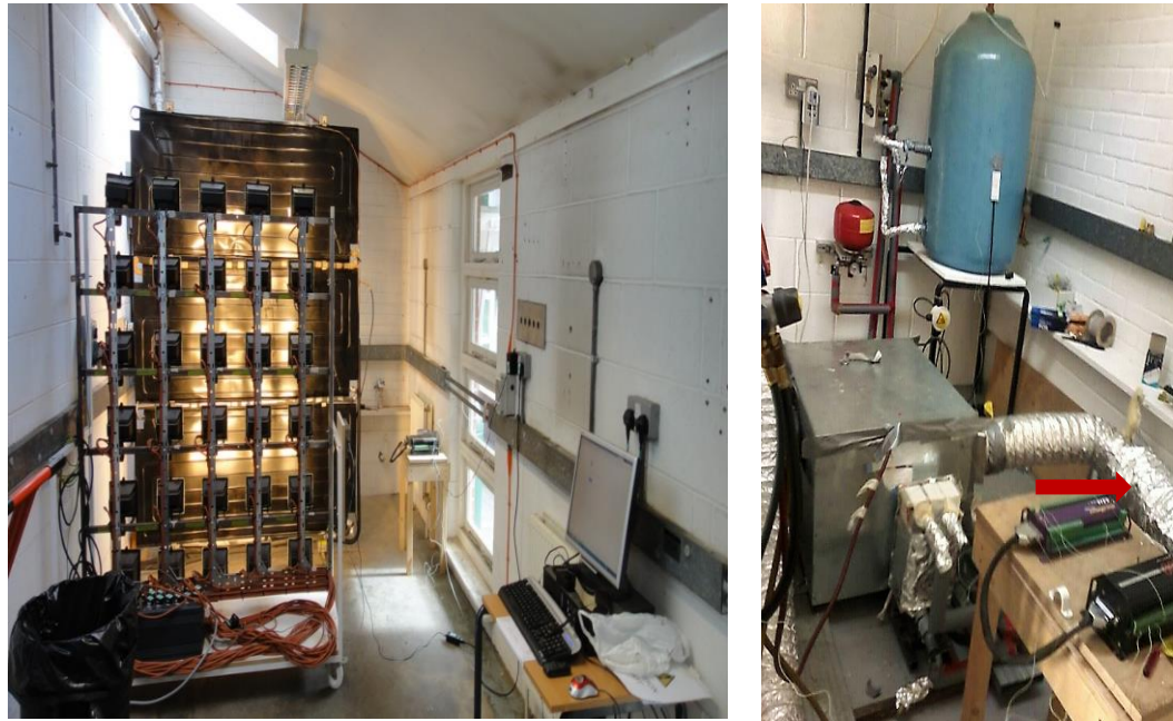
Figure 7.7. Configuration of solar simulator with evaporator/collector and DX-SAMHP set-up
