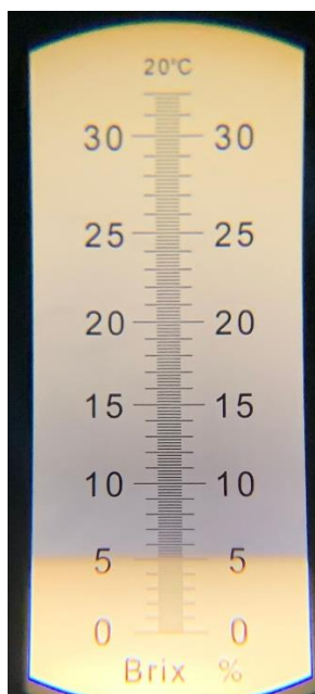
Figure 3.4. Example of a fruit Brix measurement using a handheld refractometer. The scale indicates the percentage of soluble solids content ( ^\circ\text{Bx} ) at a reference temperature of 20^\circ\text{C} . The boundary between the light and dark regions corresponds to the measured Brix value; in this example, the reading is approximately 5.2\% \text{ } ^\circ\text{Bx} , indicating the sugar concentration of the fruit juice sample.
