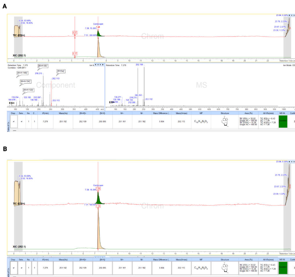
Figure 3.20: A (top): Overlaid chromatograms: TIC (ESI + , red trace) and XIC at m/z 252.1 (green, shaded) across a 24-min run on a SeQuant ZIC-pHILIC column. A single, sharp XIC peak is centered at t_R \approx 7.28 – 7.31 min and is annotated “Cordycepin.” Minor features at the solvent front ( \approx 0.34 – 0.50 min) and late elution ( \approx 23.6 – 23.8 min) are visible in the TIC but do not appear in the XIC. Ion mode: ESI + (labelled at top right). B (bottom): MS spectrum for the t_R = 7.279 min peak with automatic component assignment in ACD/Labs Spectrus Processor. Base peak [M+H]^+ = 252.109 (Mass(Amax) = 252.113), elemental formula C 10 H 13 N 5 O 3 , and Mass difference = 0.004 (Da). Additional labelled ions include 218.215 ( [M+H-34]^+ ), 246.243 ( [M+H-6]^+ ), 253.113, and a [M+Na]^+ adduct (labelled). Software confidence tile reads “Excellent.” The component table shows t_R = 7.279 min, neutral mass 251.102, [M-H]^- = 250.095 (reported), and Single XIC area = 100.00% for both ESI polarities; TIC area = 15.26% (ESI + ) and 30.02% (ESI - ) with All t_R (min) reported as TIC (ESI + ) = 7.28, XIC = 7.28, TIC (ESI - ) = 6.43, XIC = 7.29 (values as displayed in the figure). The chromatogram generated from the Thermo Exactive LC-MS employing the SeQuant ZIC-pHILIC column (Merck). The analysis was conducted over a 24-minute runtime. Visualization of the LC-MS/MS data was performed using the Spectrus Processor from ACD/Labs.
