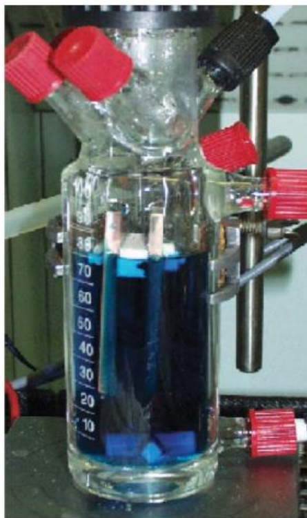
Figure 3. 1 A photo for the electrochemical cell setup being under operation for HKUST-1 preparation [178]
