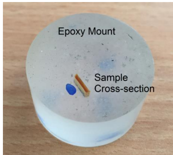
Figure 5.13: Example of printed square sample mounted into epoxy and polished for cross-sectional property characterization.
