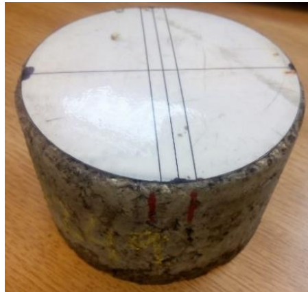
Figure 36 Template to position the deformation measurement strips
