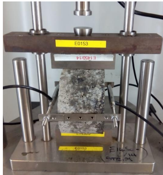
Figure 38 ITFT in strain control mode configuration
