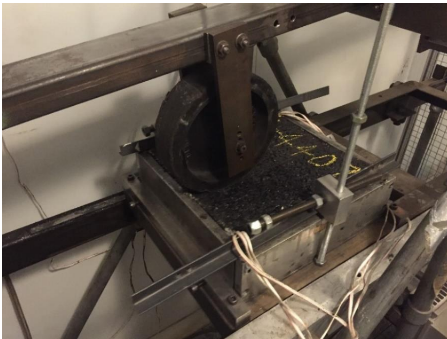
Figure 46 WTT configuration with slabs
