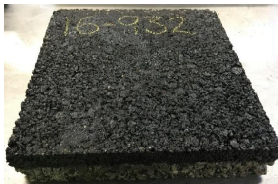
Figure 41 Slab: 30 mm cold mix + 20 mm hot mix
