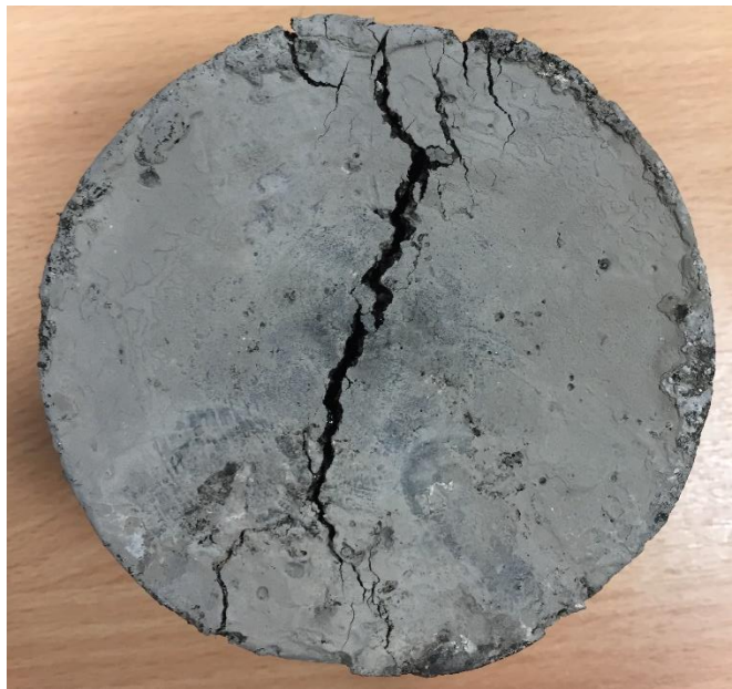
FIGURE 7 Failure in strain control mode
