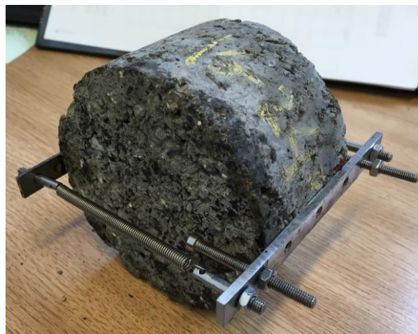
Figure 37 Deformation measurement strips glued to the specimens using a position rig
