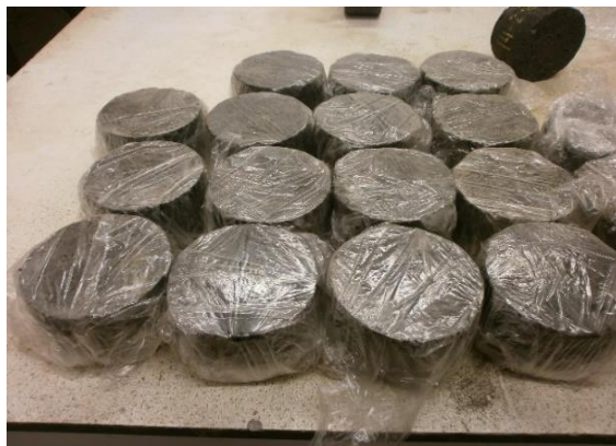
Figure 17 Double wrapped specimens for curing
