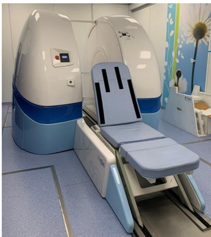
Figure 6.2: The 0.5T ASG Paramed MROpen MRI scanner at the Sir Peter Mansfield Imaging Centre at the University of Nottingham.
