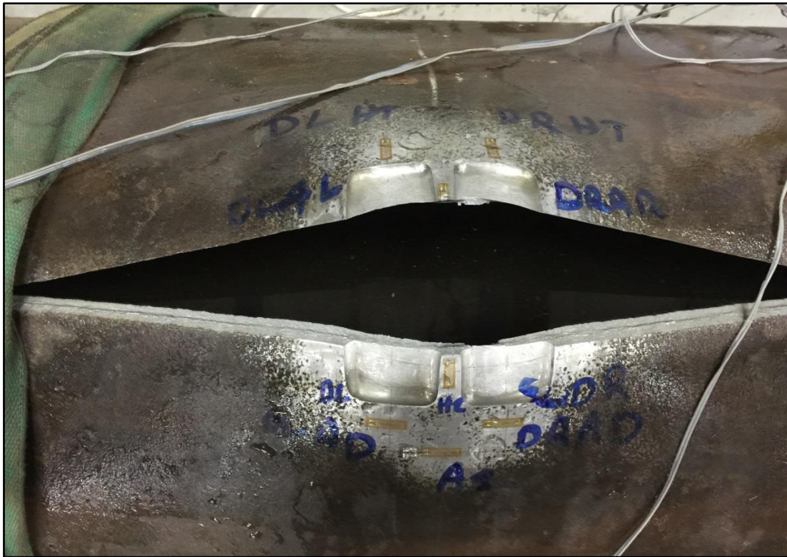
Figure 5-17: Failure of curved boxed defect spaced by 1t
