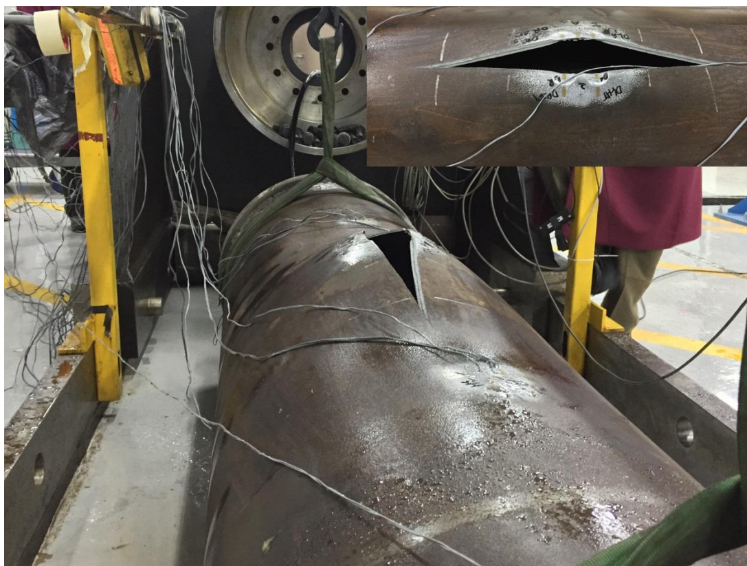
Figure 3-10: Pipe rupture image of X60 (9.5 mm) pipe with circular defects– further magnified on the top right corner.
