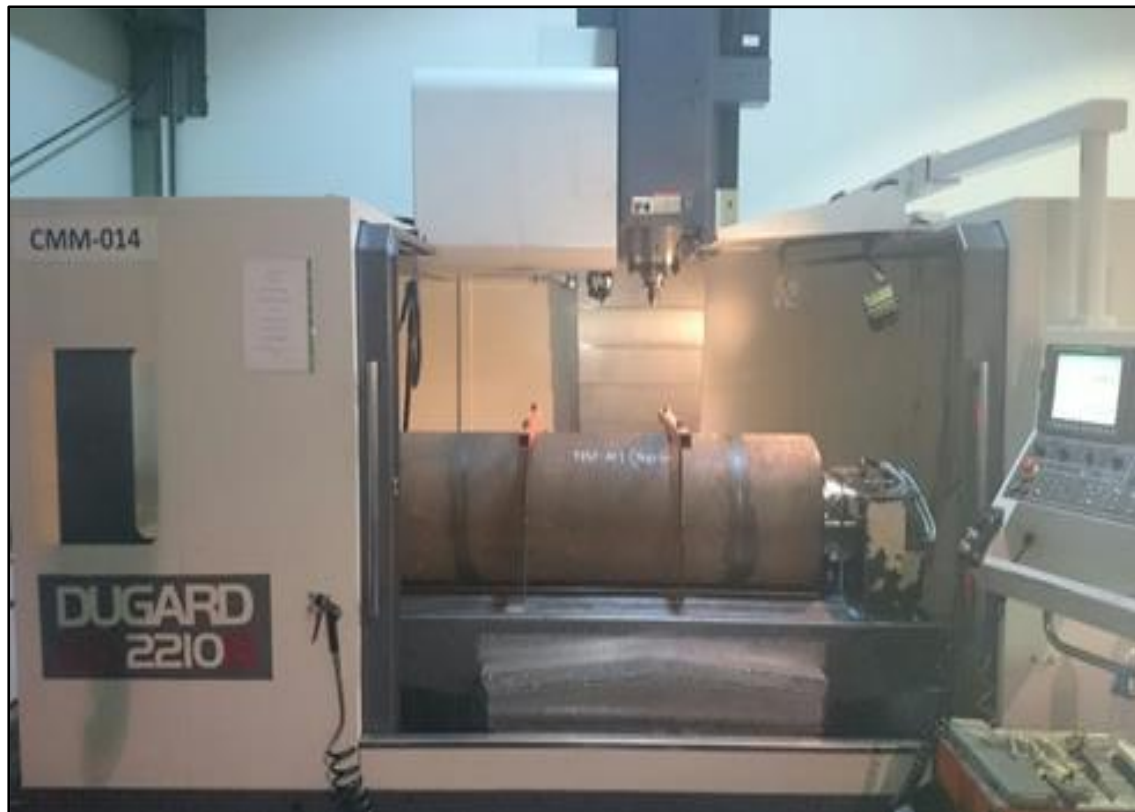
Figure 5-12: CNC machine for machining of defects
