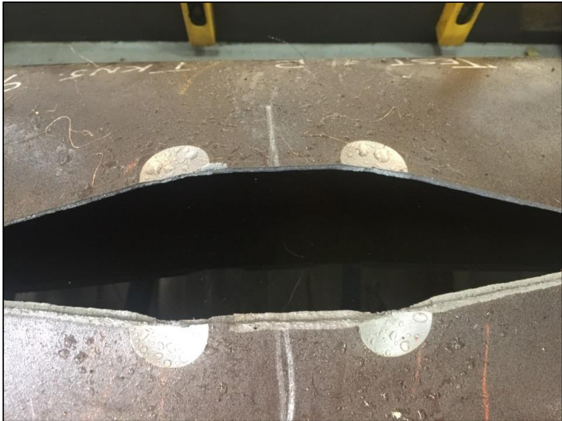
Figure 5-16: Failure of circular defects spaced by 6t.
