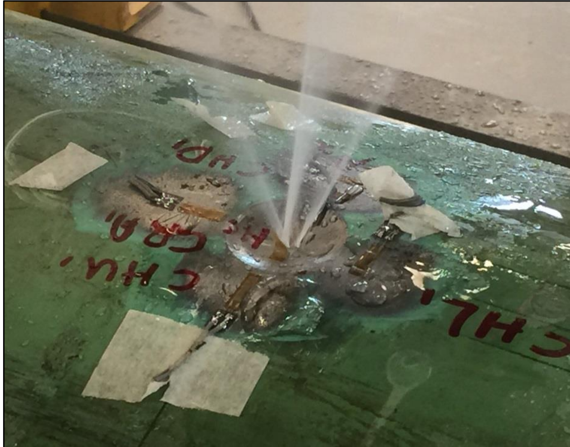
Figure 5-15: Failure of single circular defect
