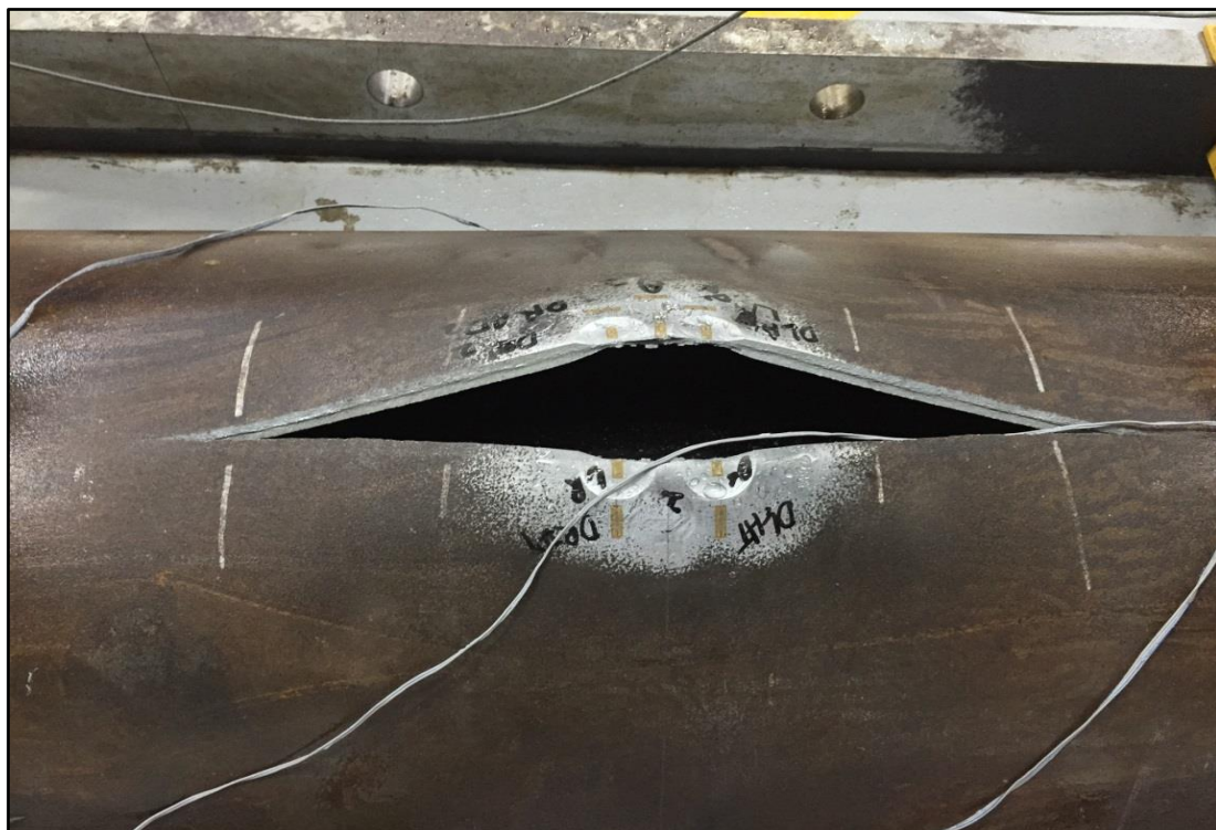
Figure 5-18: Failure of circular defect spaced by 1t
