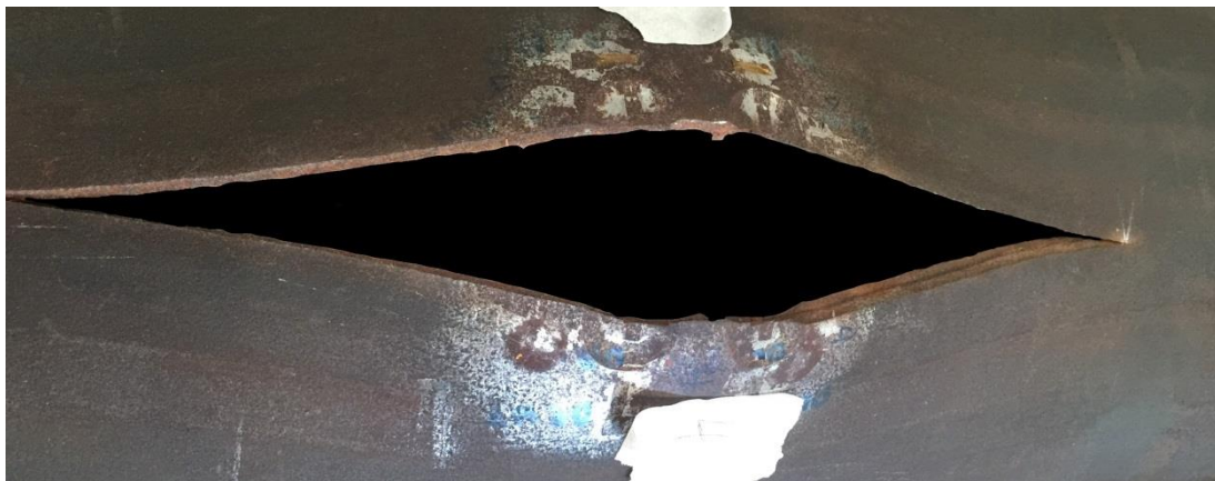
Figure 6-3: Defects failure shape (length of rupture line is 227.5 mm) for X60 pipe
