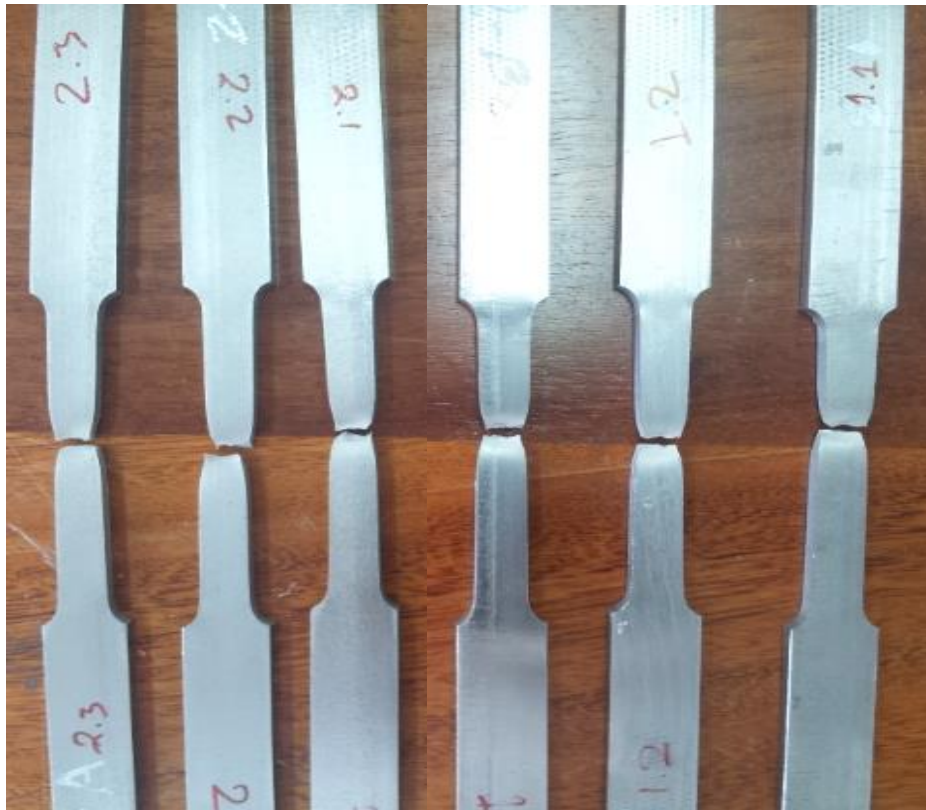
Figure 5-7: Tensile specimens of (a) X52 and (b) X60 materials after tensile tests.
